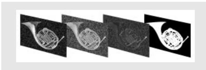
A 32-bit frame consisting of four 8-bit channels: red, green, blue, and an alpha channel mask
