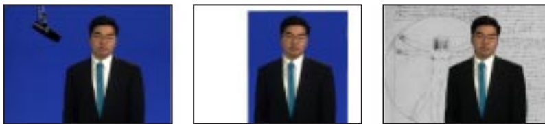
The microphone (left) is masked out by repositioning image handles in the Transparency dialog box (center), creating a garbage matte which is then keyed and composited onto a background (right).
