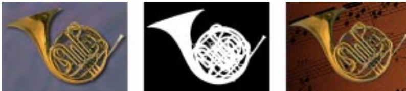
The Photoshop image (left) contains a separate alpha channel (center) which Premiere uses to composite the foreground against another background (right).
