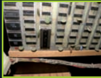
» The actual development board for Lunar Lander , with the ROMs in sockets so they could be easily changed.
