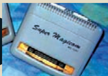
» The Super Magicom device allowed backing up of cartridge games to disk. Nintendo wasn't best pleased...
