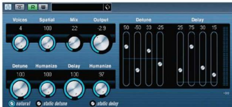
Cubase 5's Cloner plug-in creates a series of subtly varied pitch delays to add width to a vocal
