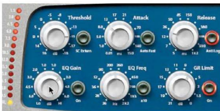
The Mpressor allows you to control parameters in the usual click and drag way but also gives you mousewheel support. Simply place the cursor over the parameter and adjust it using the mousewheel. Holding down shift puts it in to fine mode. Very useful and something more manufacturers should be doing
