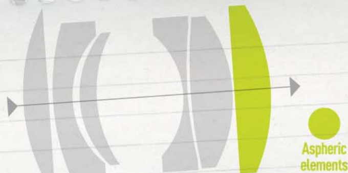
The Voigtlander Ultron 40mm f/2 'pancake' extends only 24.5mm from the camera body flange. An aspheric element reduces vignetting on full frame
