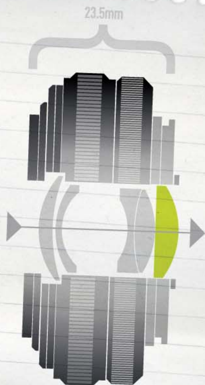
The schematic of the 25mm f/2.8 Olympus five-element pancake lens for the Four Thirds format shows the level of compression of the optical cell. Note the aspheric element used as field lens to minimise vignetting
