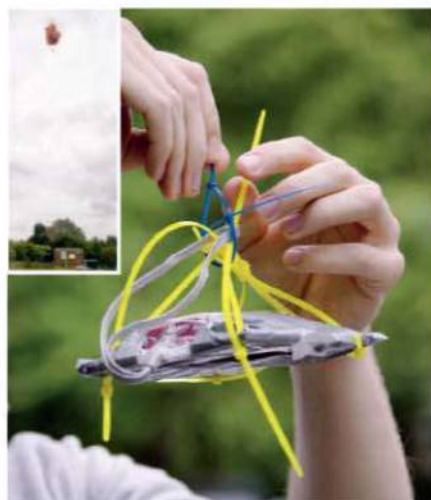
The camera was covered with a clear plastic bag and secured with tape to a piece of foam board. Cable ties were used to attach it to the balloons and kite strings. This allowed me to launch the camera to a height of nearly 30m
