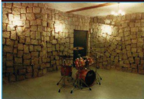
Philip Newell designed the stone live room at London's legendary Blackwing Studio. This was a very bright-sounding room and typical of many 1980s stone rooms. Note how an irregular stone pattern was used to diffuse soundwaves. Gil Norton recorded many of the guitar sounds for Trompe Le Monde by the Pixies here using close and ambient mics.
