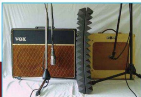
Here's how to achieve amazing separation by placing two amps close together with some absorbent material in between and close-mic'ing them. This might seem counter-intuitive at first, but it actually works surprisingly well.
