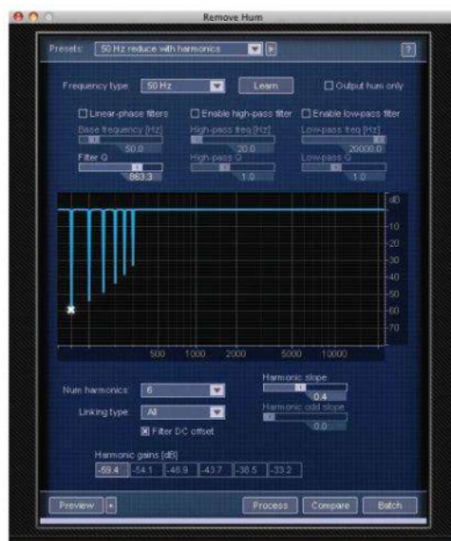
The Remove Hum tool in iZotope's RX2 can automatically calculate the harmonics from the fundamental – and have very high Q values.
