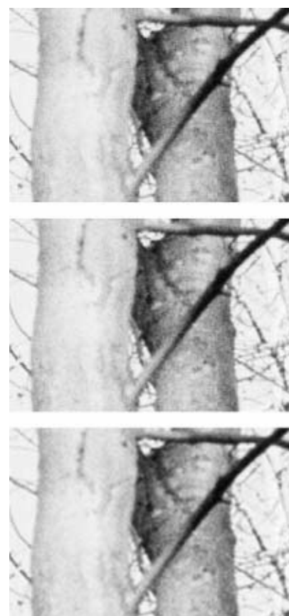
Figure 2. I scanned a TMax 100 negative at 4800, 2400, and 1200 ppi (top to bottom). Observe how much the fine detail blurs with each drop in scanning resolution. The degradation in detail is much worse than the reduction in grain; even at 1200 ppi the grain is still visible as low-contrast blotchiness, but a huge amount of detail has been lost. For the finest grain, scan at the resolution that produces the finest detail your scanner can provide.
