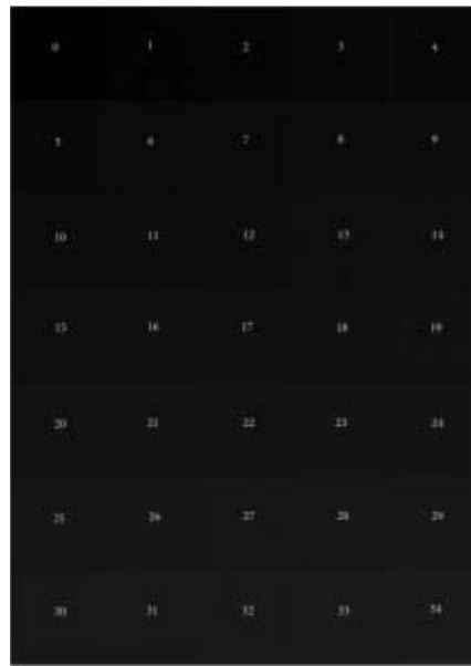
Figure 1. A test chart for measuring a printer's ability to separate tones.
