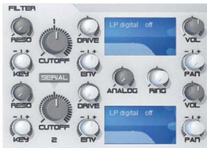
The filter on the ElectraX features an Analog knob to dial in some pleasing randomness
