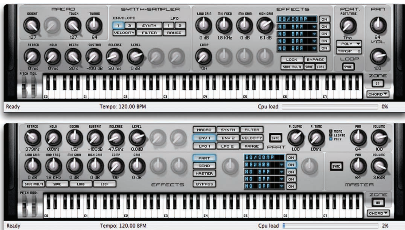
Fig. 2: The main difference between ST2.2 (top) and ST2.5 (bottom) is that the effects section has been completely revamped. It now offers three sections, each with its own bypass and up to five effects. There's also a new Master section, in which you set global Sync, Pan, and Volume.
