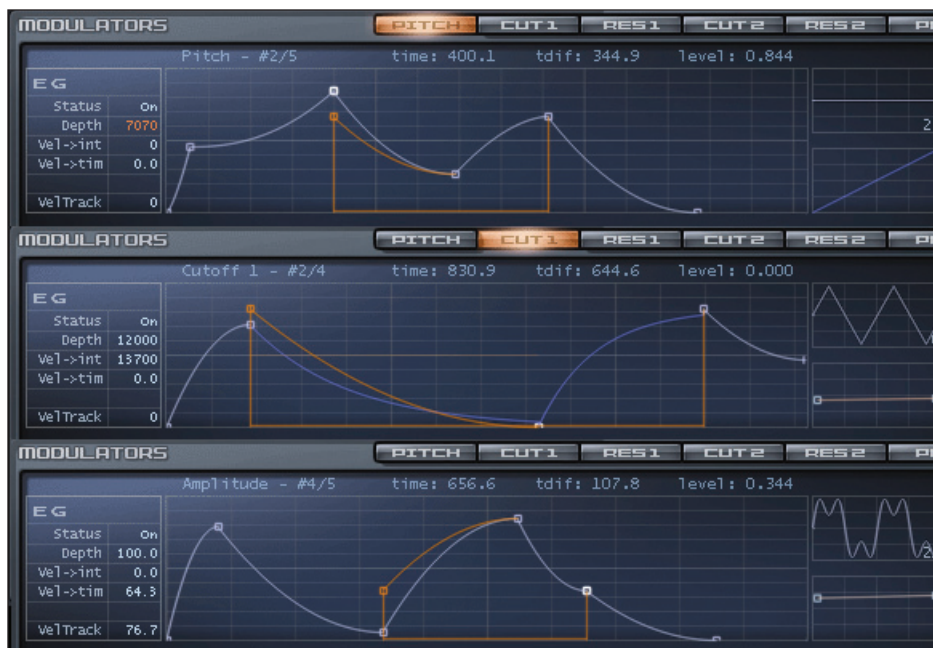
Figure 3. Rapture's envelopes support looping a segment, allowing for the creation of very sophisticated modulations. And with seven envelopes available for each of the six elements, there can be a whole lotta loopin' going on. Here three different loops modulate a single element's pitch, filter cutoff, and amplitude.
