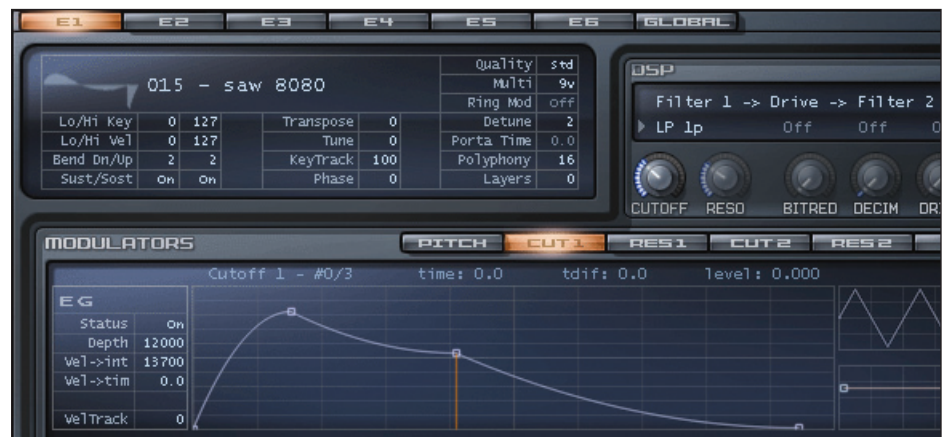
Figure 2. Envelope segments and breakpoints (nodes in Rapture) are easily programmed using click-and-drag editing. Shown here is a simple ADSR-style envelope. The vertical line under the third node indicates the sustain point.
