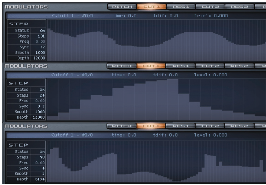
Figure 4. Complex step modulations can be drawn freely with the mouse. Shown here are the filter sweep contours for three of the six elements in our example program. Notice how large smoothing values (1000) make the first two contours sound continuous rather than stepped. The third contour, with no smoothing, jumps from value to value as the steps progress.
