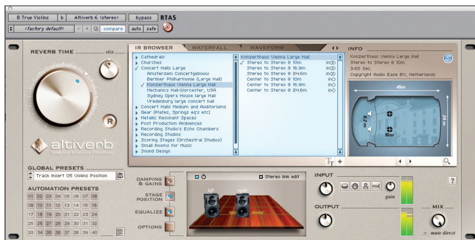
Fig. 3: The Violins Positioning program loaded into Altiverb. Its reverb tail is turned off; only the early reflections are used, and then all the instruments are sent to a common reverb program with the reverse—tails on, early reflections off. While the front-to-back positioning provides a very clear image, you might still want to use standard pan and width controls to set the left-right position more dramatically.
