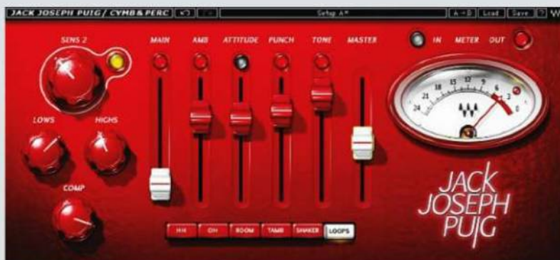
The four red central faders are essentially auxiliary returns for under-the-hood effects chains
