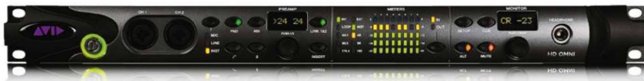
HD Omni is an "all-in-one premium sound solution" that also functions as a standalone 14x26 channel mixer
