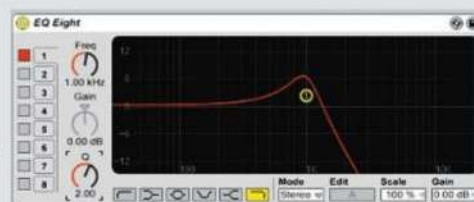
A low-pass filter with resonance in Ableton Live. The graph shows us the filter's frequency response - note the peak around the cutoff due to the cranked resonance
