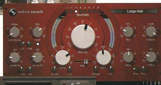
112dB's Redline Reverb is a true stereo algorithmic reverb plug-in unit
