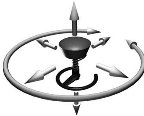
Fig. 5.3 The ChairIO's DOFs using the Swopper™ as underlying chair
