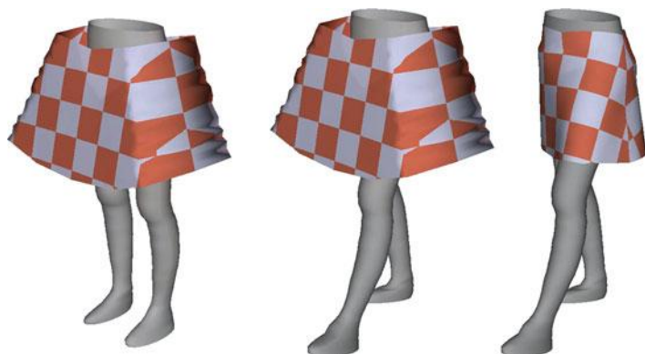
Fig. 7.2 Determining the configuration of the skirt-model compound in the first frame is split into three steps. The initial configuration is manually determined on the undeformed model, the model is deformed, and the cloth is draped on the legs
