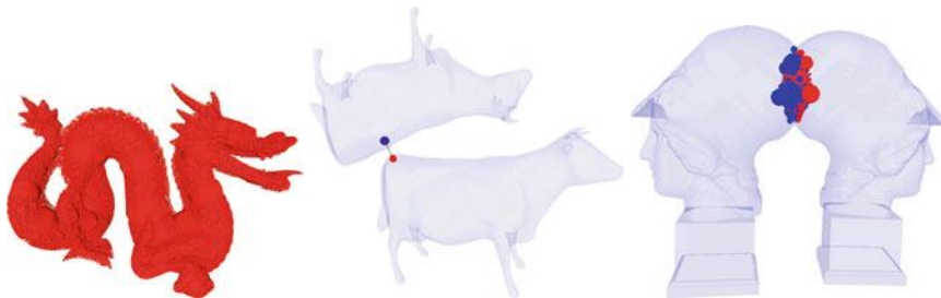
Fig. 10.1 Our Inner Sphere Trees are based on sphere packings of arbitrary polygonal objects ( left ). They are suitable for different kinds of geometric queries, namely proximity queries ( middle ) and our new method for computing the penetration depth, the penetration volume ( right )
