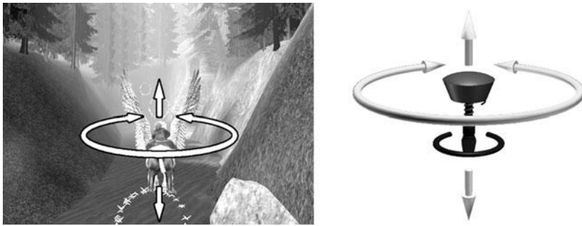
Fig. 5.5 Bird flight controlled with the ChairIO. The left image shows the game with the indicated ways of navigation: orientation and wing beat. The right image shows the corresponding illustration of the parameters on the ChairIO
