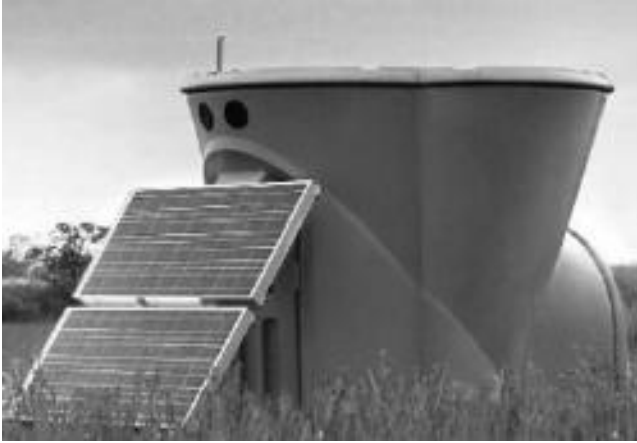
FIGURE 6-17 Picture of the Nomad™ SODAR unit. Size of the unit is 2 m × 2 m × 2 m and weighs between 350 and 450 kg. (Photo (copyright) Justin Arcangeli. Courtesy Second Wind Inc.)
