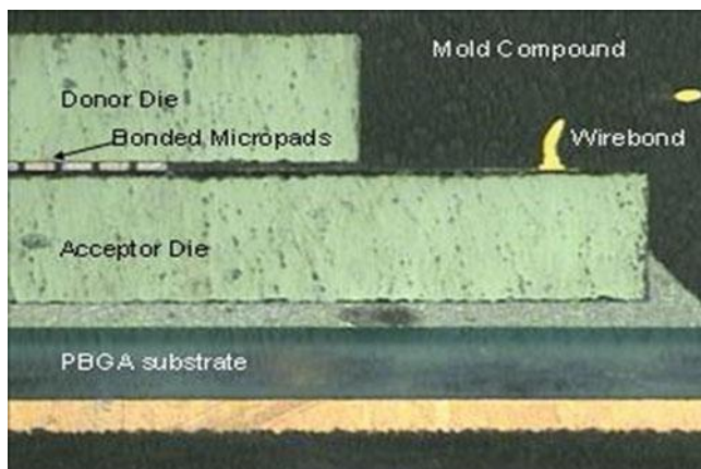
Fig. 15.14 Cross-section of a packaged single stack assembly [2]
