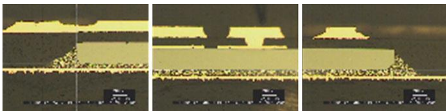
Fig. 15.8 Embedded die in a resin-coated copper (RCC) layer with thermally conductive adhesive
