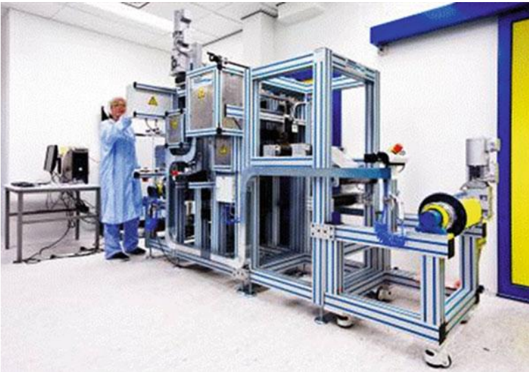
Fig. 13.3 R2R lamination line (at Holst Centre, Eindhoven)
