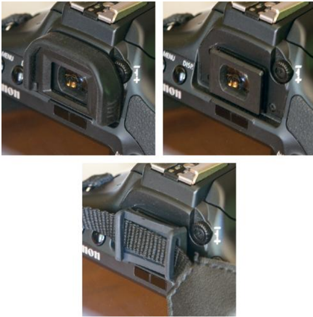
Figure 6-27. To use the eyepiece cover, first remove the eyepiece. Fit the eyepiece cover (attached to the strap) over the eyepiece mount. When you're done, replace the eyepiece.
