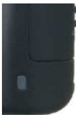
Figure 2-6. This lamp lights up whenever the camera is writing to the card. Removing the media card while this lamp is lit could wreck the images stored on the card.
