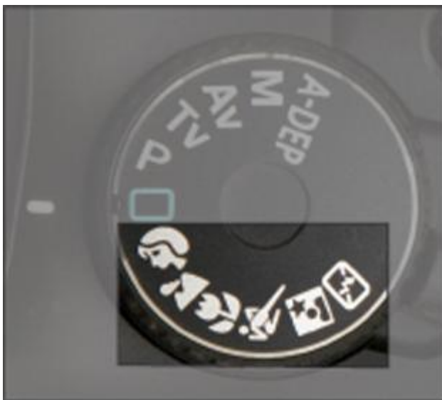
Figure 1-11. These options on the Mode dial are scene modes, which bias the camera's decisions under specific conditions so that it calculates more appropriate exposures.
