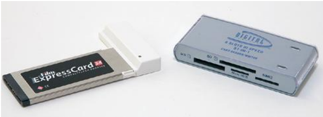
Figure 4-2. On the left is a CardBus card reader that can plug directly into a CardBus slot on a laptop. On the right is a card reader that plugs into a USB 2 slot. Note the huge number of card formats that it supports.
