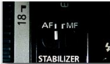
Figure 1-6. Your lens should have a way to change from auto to manual focus. If the lens provides stabilization, there will be a switch for turning stabilizing on and off.
