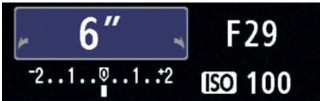
Figure 7-23. The XS offers shutter speeds up to 30 seconds long (longer if you use Bulb mode). Here it's indicating a six-second exposure.
