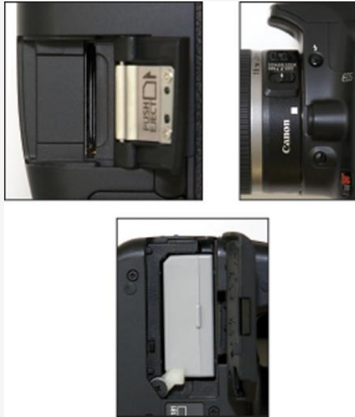
Figure 1-1. From left to right, the Rebel XS's media slot, lens mount button and reference dot, and battery.
