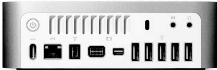
Figure 2-5: The Mac mini's back, showing cable con- nections.
