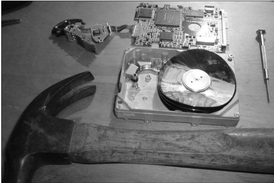
Figure 6-2: Dis- assembled hard drive with bent disks.
