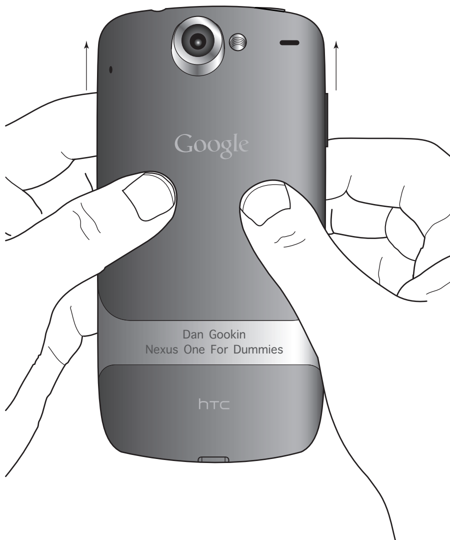
Figure 1-1: A thumb placement suggestion for removing the back cover.
