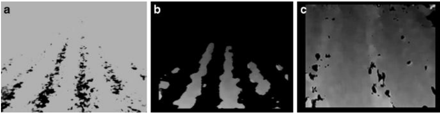
Figure 5.41 Exposure-based segmentation for identifying crop rows in disparity images: (a) aperture-biased initial image; (b) corresponding disparity map; (c) conventional disparity image obtained when the lens aperture is set for normal use
