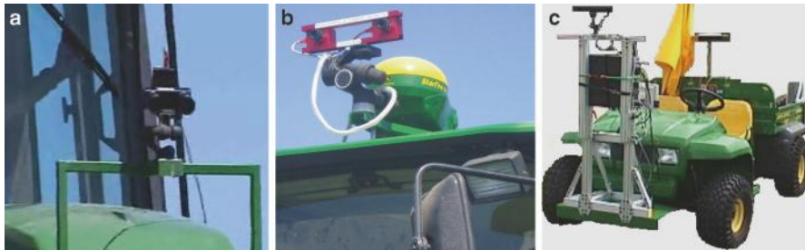
Figure 5.8 Alternative positions for stereo cameras on intelligent vehicles: (a) purpose-built frame; (b) center of the cabin; (c) front of vehicle
