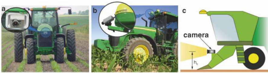
Figure 4.9 Camera locations: (a) front end of tractor nose; (b) tractor cabin; (c) harvester header
