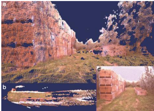
Figure 5.53 Detection of a static obstacle in an orchard: (a) 3D virtual representation of scene; (b) field map; (c) actual scene
