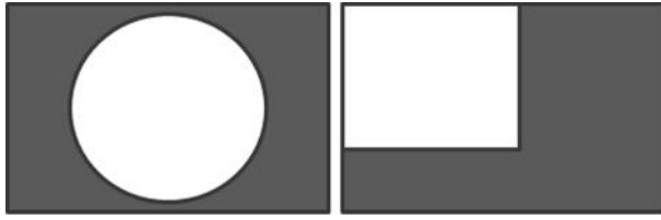
Figure 5.15 Low-pass filters for different frequency transforms: (a) DFT; (b) DCT
