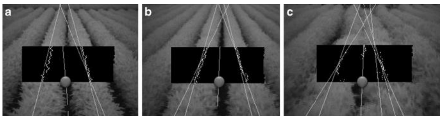
Figure 4.30 Multiple lines detected as estimates of the two central tracking rows: (a) three lines; (b) four lines; (c) five lines
