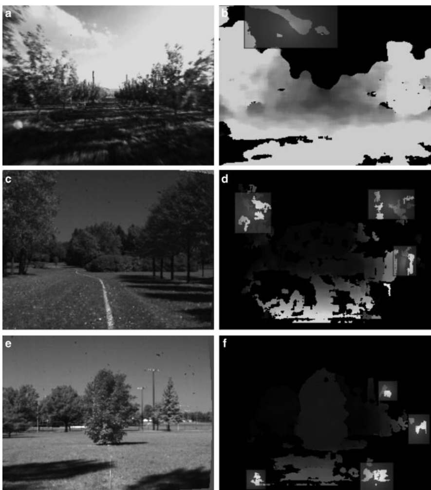
Figure 5.13 Actual (a, c, e) and disparity (b, d, f) images carrying mismatching pixels
