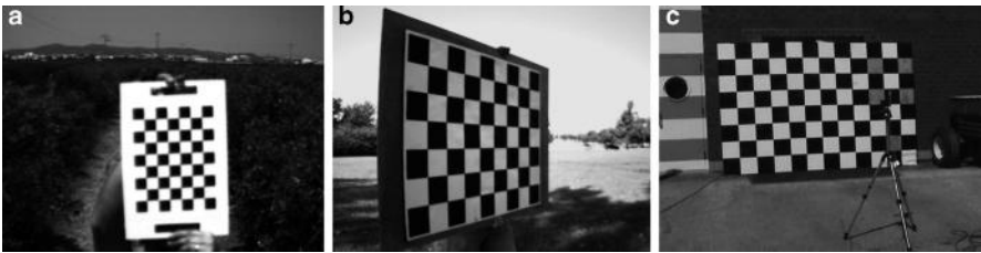
Figure 5.7 Calibration boards used for stereo cameras: (a) small board; (b) medium-sized board; (c) large board
