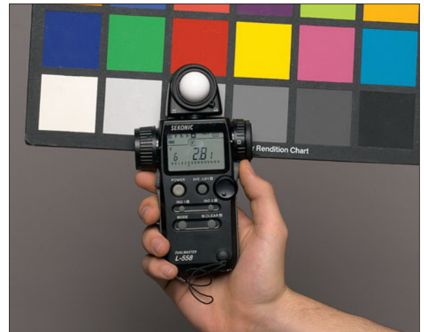
Figure 2.12 A hand-held spot meter allows you to take a reading of a small 1° angle of view for an accurate reading of a single patch on the ColorChecker Target.
