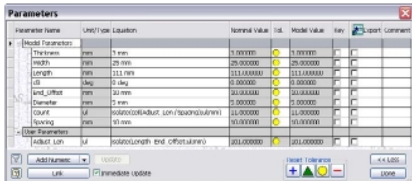
FIGURE 5.46 Formulas to adjust the hole spacing
