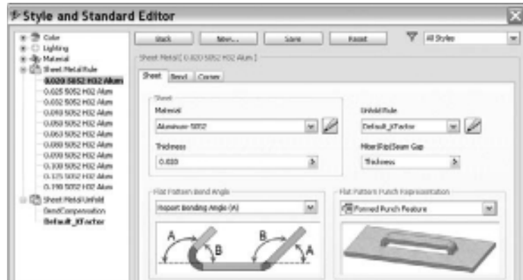
FIGURE 6.26 Style And Standard Editor dialog box, Sheet Metal Rule page displaying active rule
