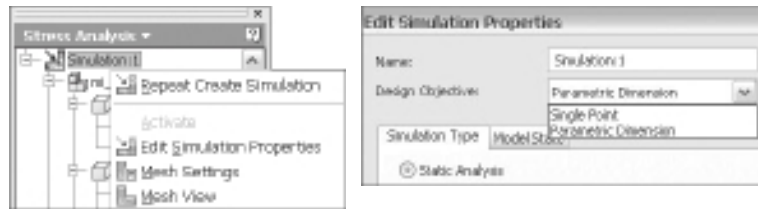
FIGURE 17.13 Setting a simulation to the Parametric Dimension design objective
