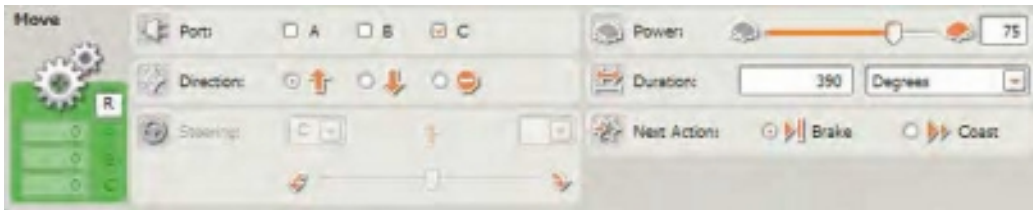
Figure 12-23. The false path MOVE block's configuration panel
