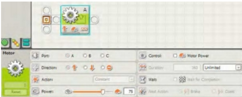
Figure 24-1. The MOTOR block and its configuration panel
