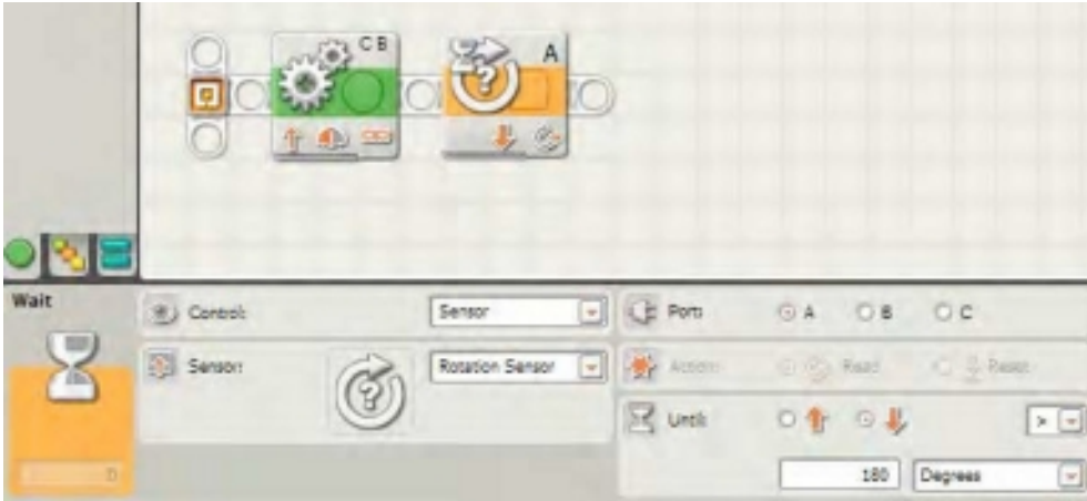
Figure 10-7. The ROTATION SENSOR WAIT block and configuration panel
