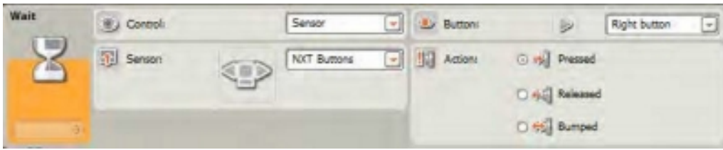
Figure 24-12. The second WAIT block's configuration panel
