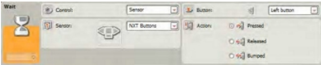
Figure 24-8. The first WAIT block's configuration panel
