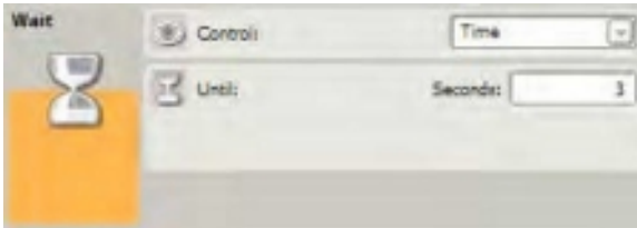
Figure 21-5. The first WAIT block's configuration panel
