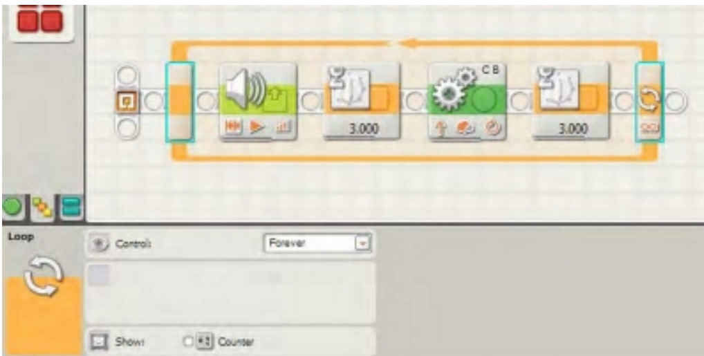
Figure 21-3. The complete program and the LOOP block's configuration panel
