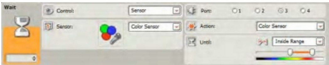
Figure 12-20. The COLOR SENSOR WAIT block's configuration panel
