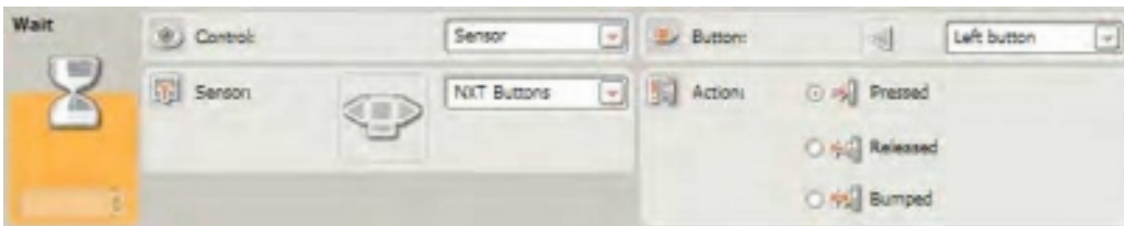
Figure 19-13. The NXT BUTTON WAIT block's configuration panel
