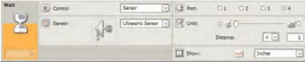
Figure 10-19. The ULTRASONIC SENSOR WAIT block's configuration panel
