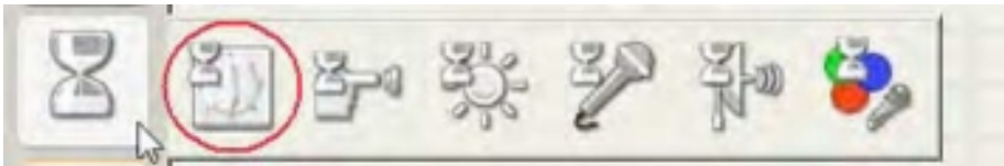
Figure 3-6. Adding a WAIT block will allow you to view the “Hello World!” text.
