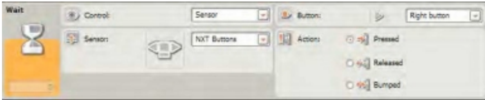
Figure 15-23. A final NXT BUTTON WAIT block keeps the program from ending.
