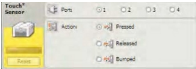
Figure 9-4. The RIS Touch sensor's configuration panel
