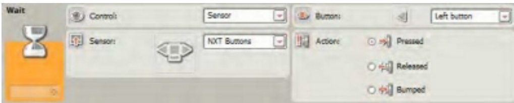
Figure 22-22. THE WAIT block's configuration panel
