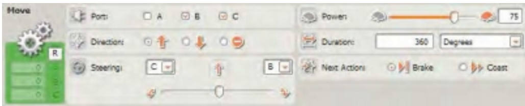
Figure 20-10. The second MOVE block's configuration panel
