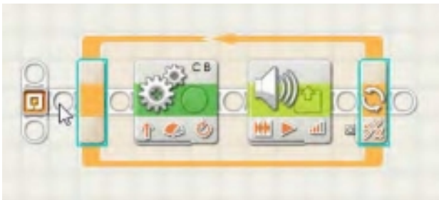
Figure 11-17. Create a new beam by starting at the beginning of the existing beam.
