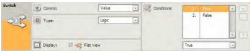
Figure 15-20. The SWITCH block's configuration panel.
