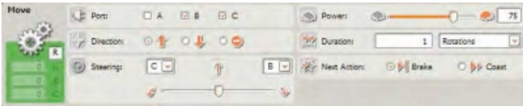
Figure 21-6. The MOVE block's configuration panel
