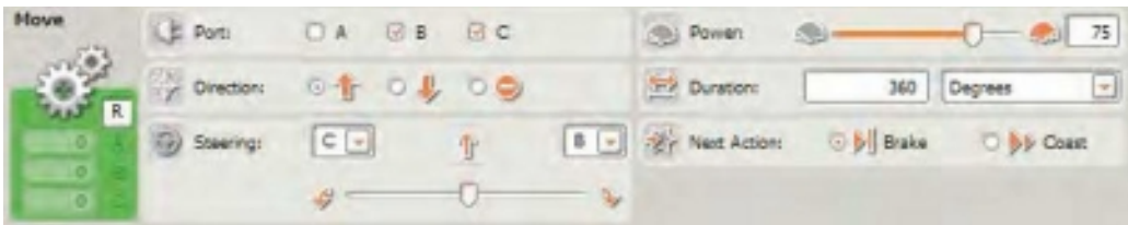
Figure 20-7. The first MOVE block's configuration panel
