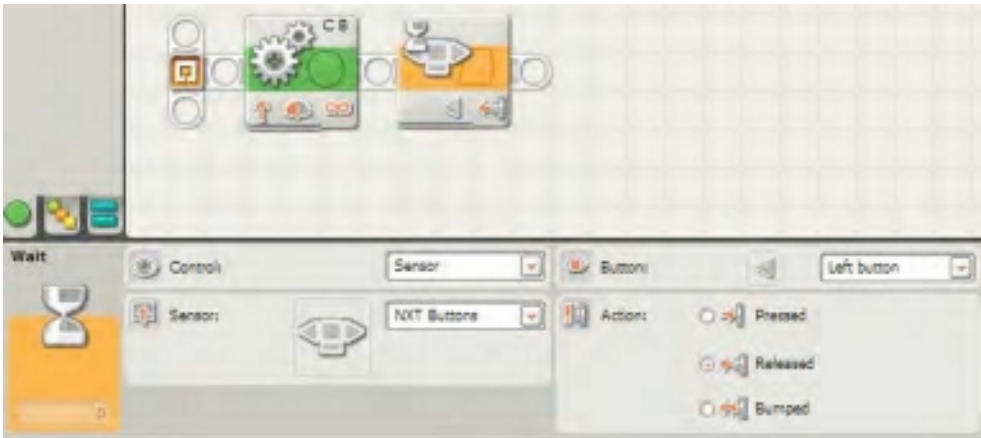
Figure 10-6. The NXT BUTTONS WAIT block and configuration panel
