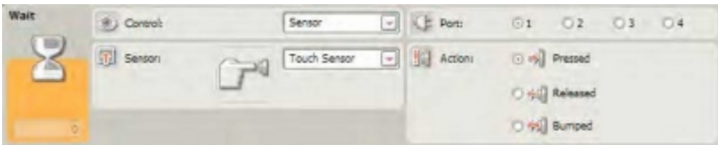
Figure 10-22. The second TOUCH SENSOR WAIT block's configuration panel
