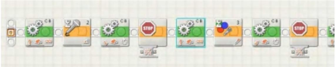
Figure 13-5. Use a series of STOP blocks when testing a long program.
