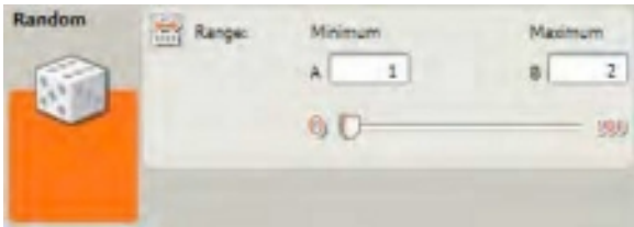
Figure 22-10. The RANDOM block's configuration panel.
