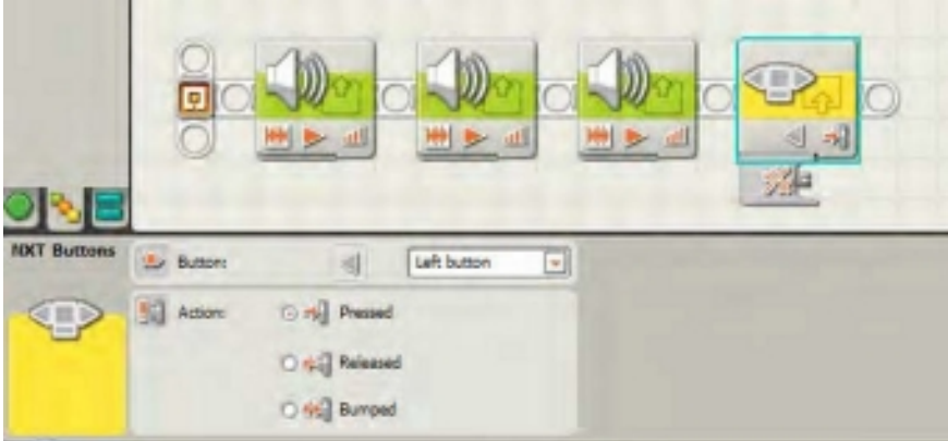
Figure 18-12. The NXT BUTTONS SENSOR block will monitor the Left button.
