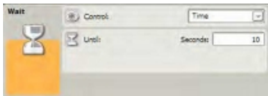
Figure 4-14. The WAIT TIME block configuration panel
