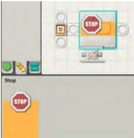
Figure 13-1. The STOP block and its configuration panel
