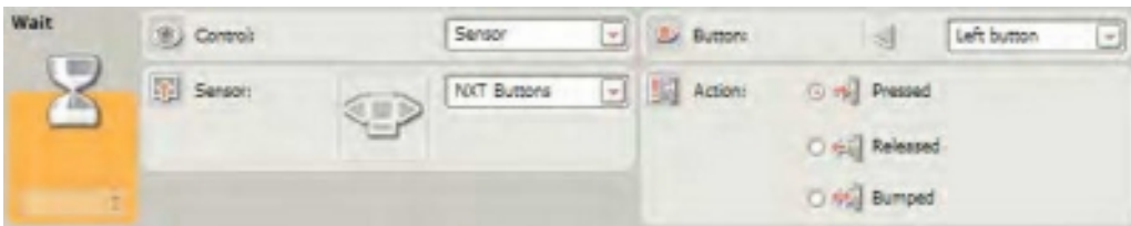
Figure 20-14. The NXT BUTTONS WAIT block's configuration panel
