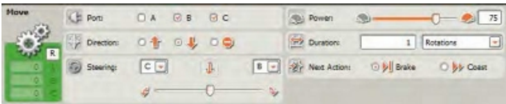
Figure 22-12. The MOVE block's configuration panel for condition 2
