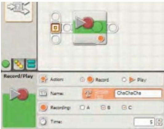
Figure 5-9. A single RECORD/PLAY block is required to record a movement.
