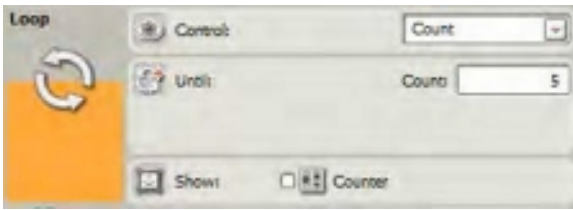
Figure 22-9. The LOOP block's configuration panel
