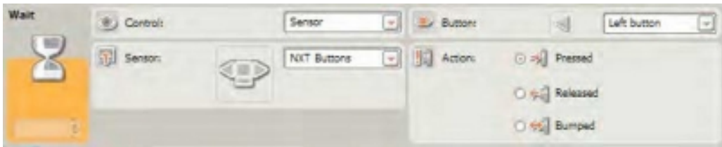
Figure 16-23. The NXT BUTTON WAIT block's configuration panel
