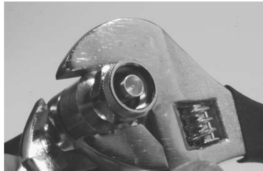
FIGURE 5-37 LMR600 using EZ-Connector Step 2: lock the two parts in place using crescent wrenches.
