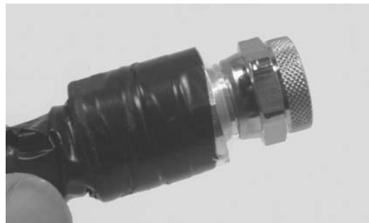
FIGURE 5-39 LMR600 using EZ-Connector Step 4 – always weatherize.
