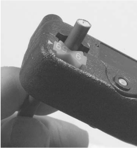
FIGURE 5-20 Use an LMR195/RG58 stripping tool to begin termination (this tool also works well with Ethernet cables).
