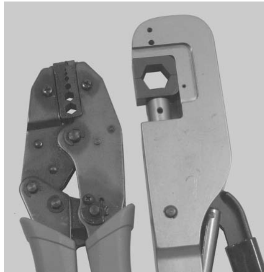
FIGURE 5-19 The required crimping tools. Left: for LMR195/RG58 and the SMA connectors; right: for LMR600 and the N-type connectors.
