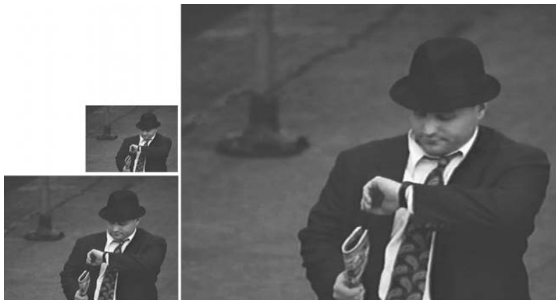
FIGURE 2-7 The picture at the upper left is using the existing CIF bits ( 352 \times 240 ) and the image on the lower left is using existing 4CIF bits ( 704 \times 480 ) converted to 300 dpi (shrinks the image to about one-quarter the size on screen). The picture on the right shows the same frame capture, following the previous tips for upscaling using Adobe Photoshop CS3, an Nvidia 9500GT, and a 1-GB video graphics card on a 19-inch LCD monitor at 1280 \times 1024 resolution.
