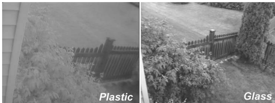
FIGURE 3-6 Plastic versus glass lenses.
