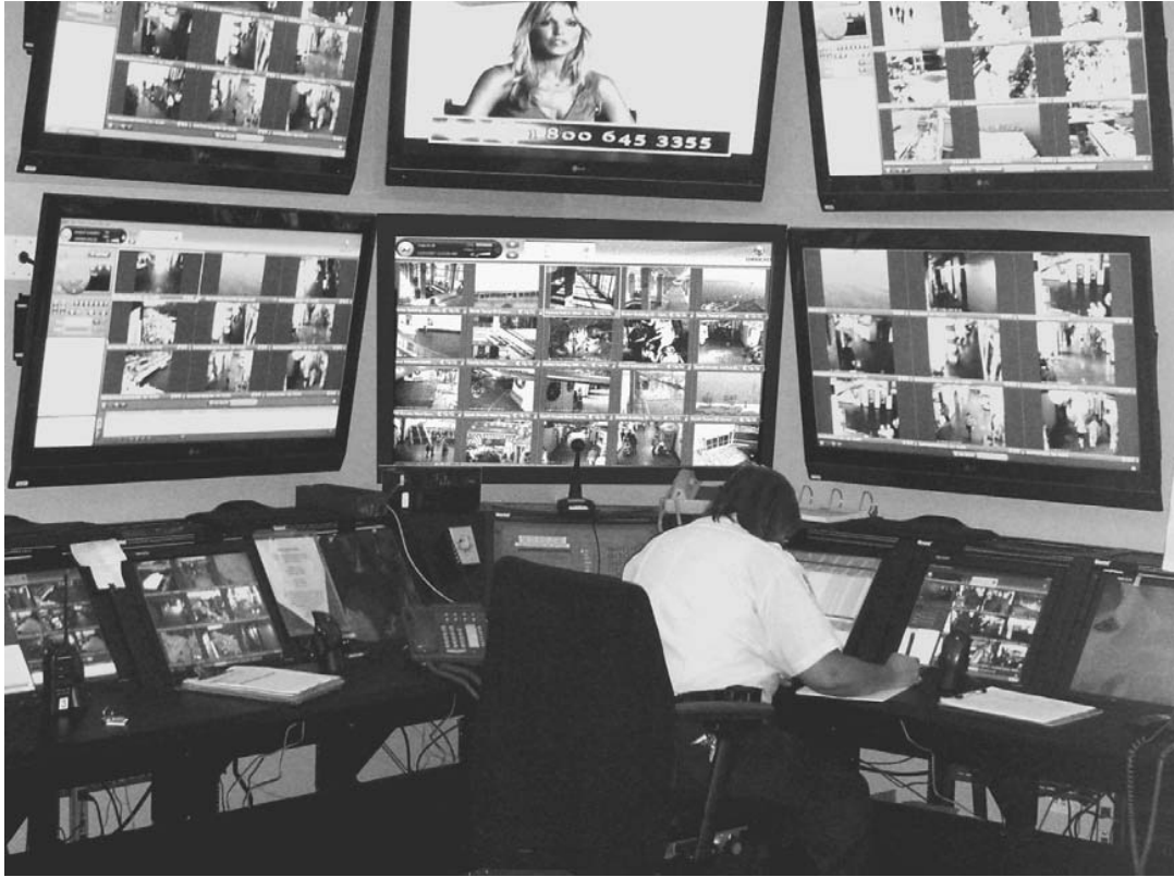
FIGURE 8-2 Navy Pier Command Center uses two dual monitor Nvidia video cards to link four 46" LCD monitors per workstation (photo courtesy of Tim Herlihy and Navy Pier).
