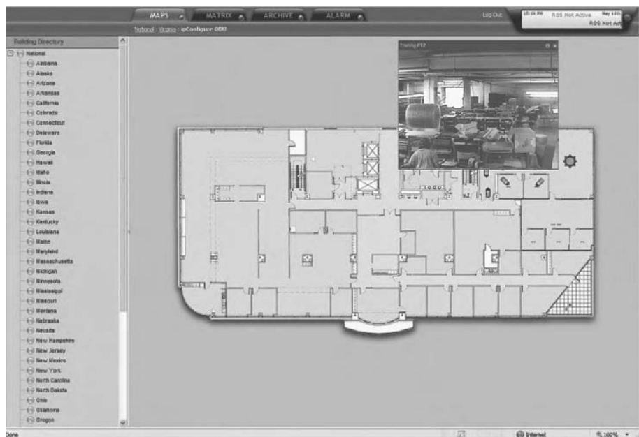
FIGURE 7-6 Most professional VMS software suites now include mapping solutions. IpConfigure also offers a mapping solution with live streaming video as a pop-up when scrolling over a camera icon.
