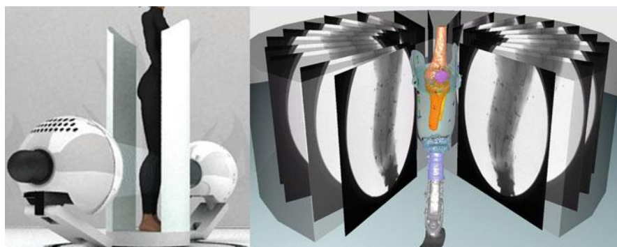
Fig. 5 (a) (Left) The DRSA turntable digital radiography scanner (see also Fig. 1 in use) and (b) (right) the axisymmetric cone-beam stack of image sequences that can be reconstructed during post-processing by registering the DRSA X-ray system in 3D, using the projection data [31, 39]
