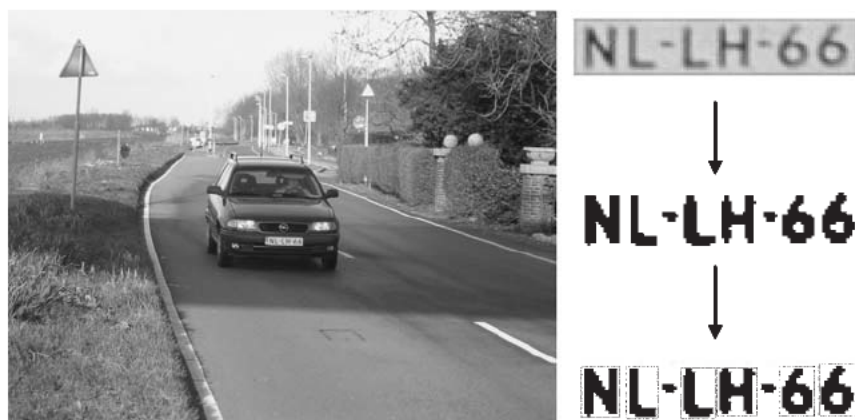
Figure 1.1 License plate recognition: a classification problem with noisy measurements
