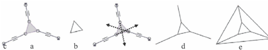
Figure 3. Constructing the MLG for a 3 RPR manipulator.
