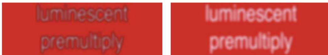
Figure 3.30 Did you create edge multiplication by luma matting a layer against black with itself (left)? Luminescent Premultiply (right) fixes this.
