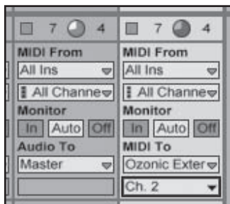
Figure 7.7 The MIDI track on the left has an instrument loaded. Notice that the bottom menu in this track is labeled Audio To, indicating that this track now outputs audio. The track on the right does not have an instrument loaded, so it still outputs MIDI.
