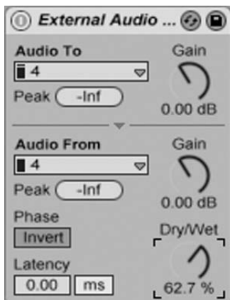
Figure 9.33 The External Audio Effect shown above will route audio through whatever hardware is connected to input and output #4 on your audio interface.
