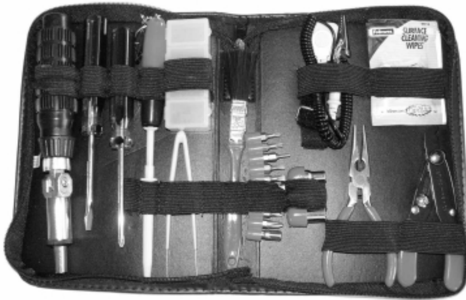
Figure 4-2. Toolkit with anti-static strap and pliers.
