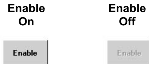
Figure 10.11 Enable property can deactivate a control.
