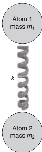
Figure 9.5. Illustration of a diatomic molecule with the two bonding atoms connected by a massless spring with force constant \kappa .
