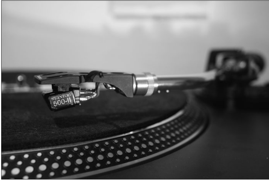
Figure 6-4: The tonearm perfectly balanced, with the needle removed from the cartridge to avoid damage.
