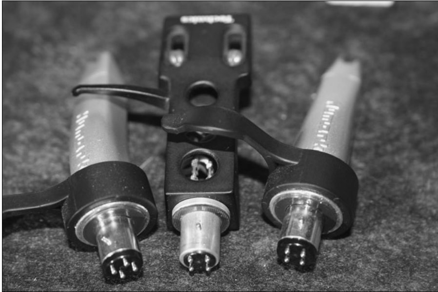
Figure 7-1: The same connection on the back of different cartridges.
