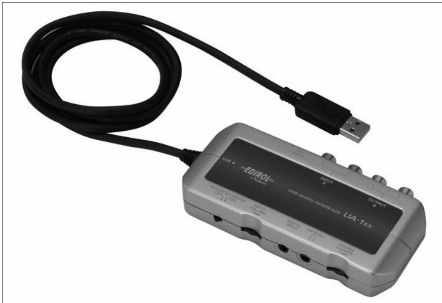
Figure 13-4: The Edirol audio to USB by Roland with analogue inputs and outputs connected to a USB connection.
