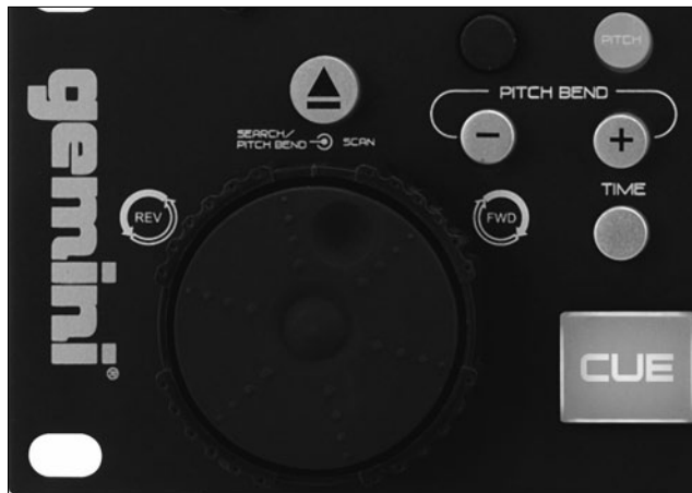
Figure 8-5: The jog dial on a twin CD deck.
