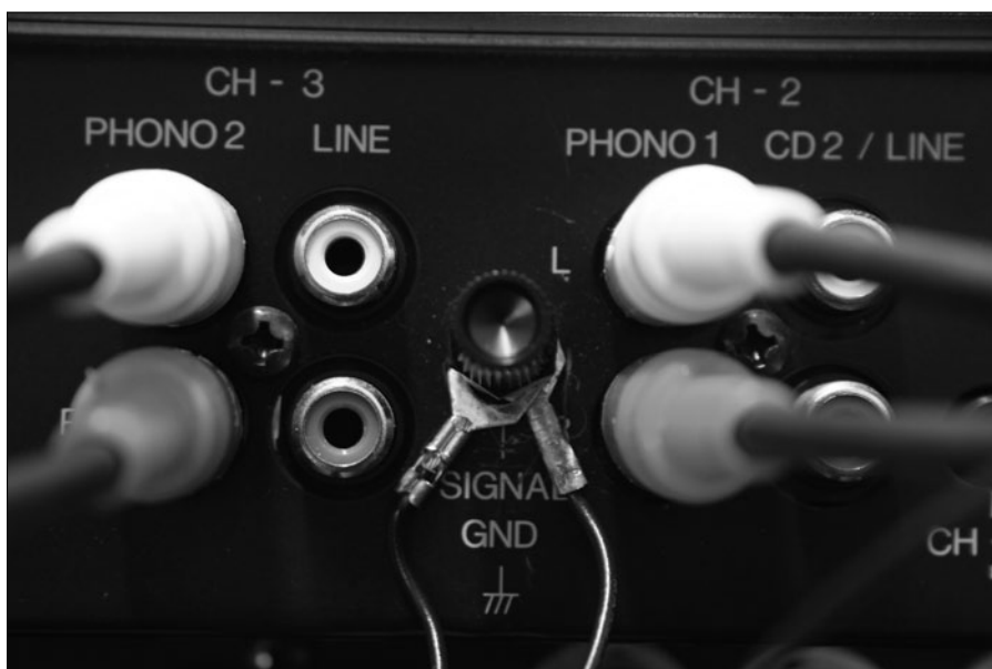
Figure 13-3: Two ground wires screwed to the back of the mixer.
