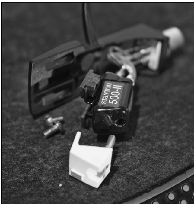
Figure 7-3: A disassembled needle and car- tridge with a Technics headshell.
