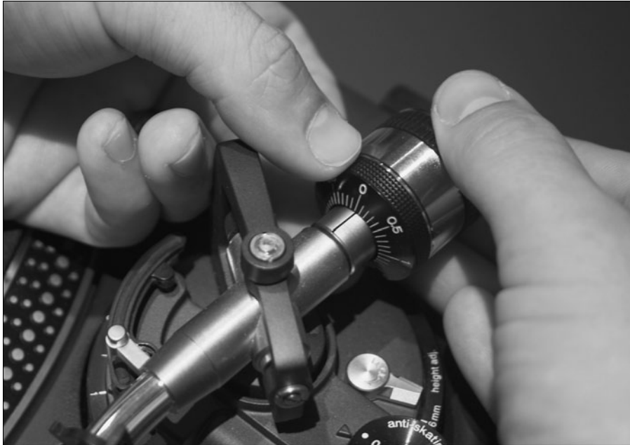
Figure 6-5: One hand supports the back of the counterweight while the other rotates only the numbered ring.
