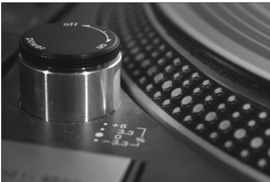
Figure 3-1: The power switch on a turntable, with the strobe light underneath it shining onto the calibration dots on the deck platter.
