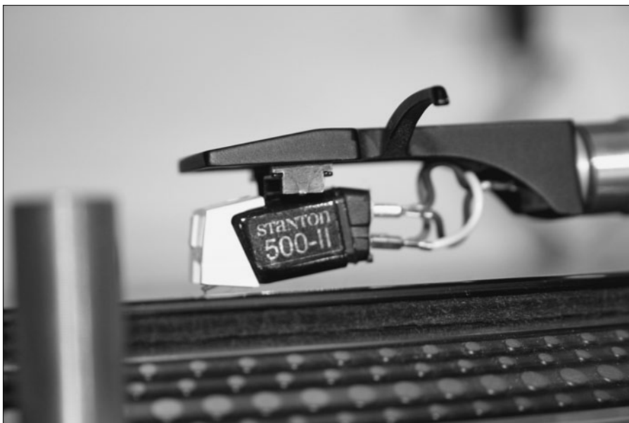
Figure 7-2: A Technics headshell with Stanton 500AL attached.
