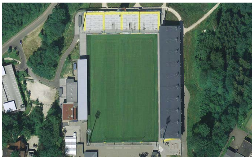
Fig. 7.1-32 Aalen, Germany, Orthophoto of the stadium 1:1000, altitude 1.2 km, GSD 12 cm
