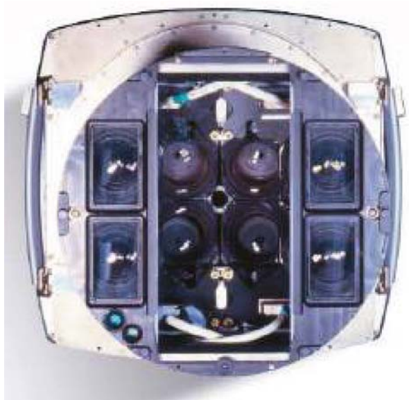
Fig. 1.5-2 The DMC as seen from below. The four inner cameras generate the panchromatic image (Z/I Imaging, 2003)
