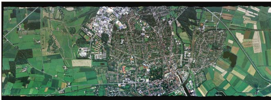
Fig. 7.1-29 Aalen, Germany, Image strip 1:35,000 for sensor calibration, altitude 1.2 km, GSD 12 cm
