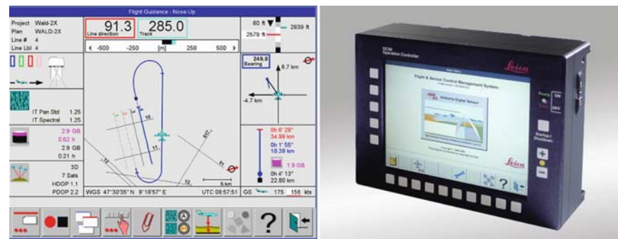
Fig. 7.1-16 New FCMS (Flight & Sensor Control Management System) incl. Flight Guidance and the Pilot and Operator Controller OC50 for FCMS
