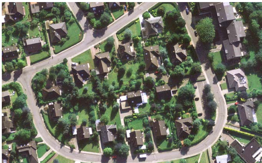
Fig. 7.1-31 Aalen, Germany, Orthophoto 1:1000 (zoom of 7.1-29), altitude 1.2 km, GSD 12 cm
