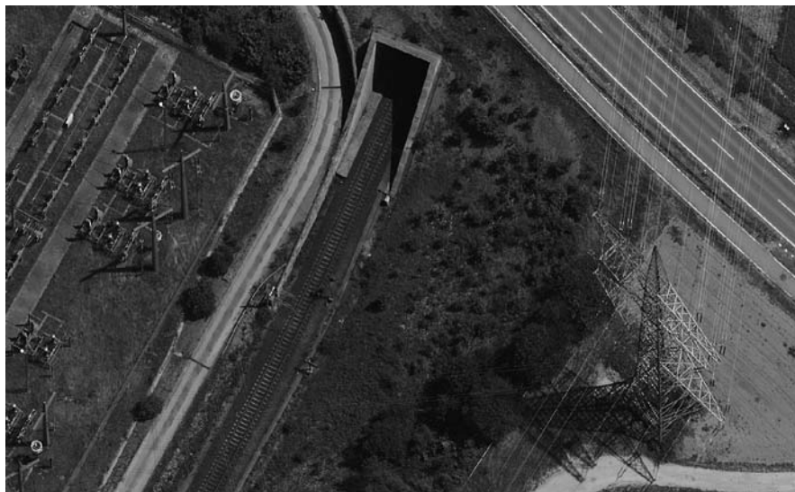
Fig. 7.1-22 Vaihingen, Germany, Orthophoto 1:500, altitude 0.5 km, GSD 5 cm
