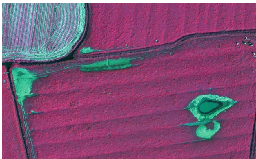
Fig. 7.1-36 Eiderstedt, Germany, False-colour orthophoto for the update of biotopes 1:1000 (zoom of 7.1-35), altitude 2.0 km, GSD 20 cm
