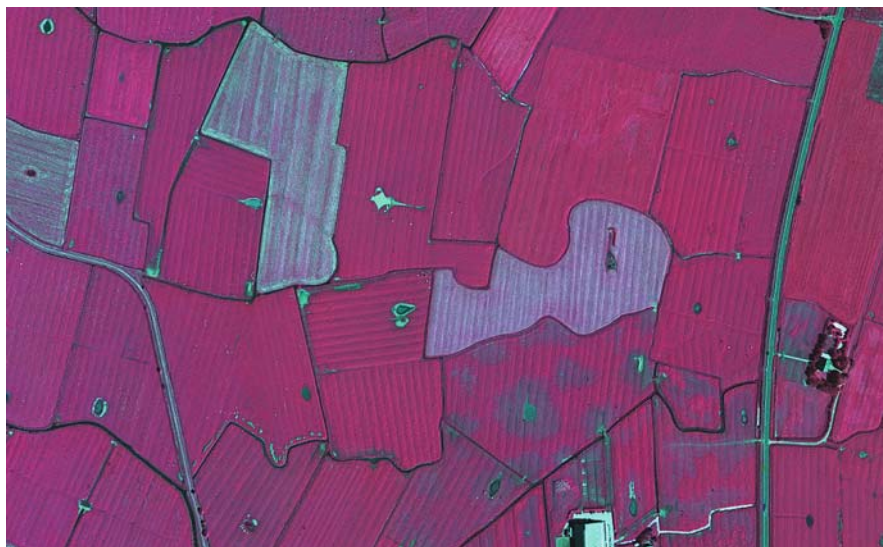
Fig. 7.1-35 Eiderstedt, Germany, False-colour orthophoto for the update of biotopes 1:2500, altitude 2.0 km, GSD 20 cm
