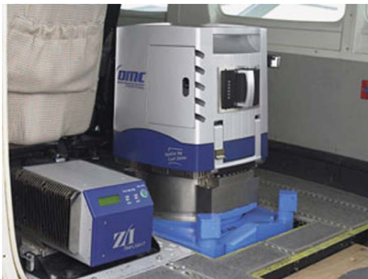
Fig. 7.2-1 DMC camera located in a T-AS gyro stabilized mount
