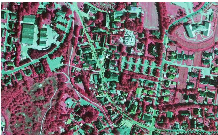
Fig. 7.1-34 Eiderstedt, Germany, False-colour orthophoto for the update of biotopes 1:5000, altitude 2.0 km, GSD 20 cm
