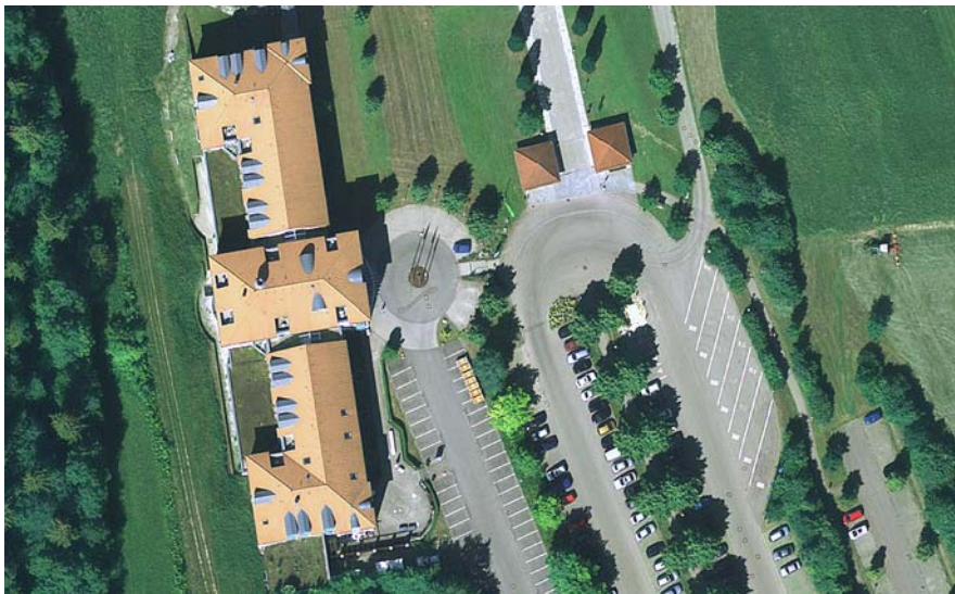
Fig. 7.1-33 Aalen, Germany, Orthophoto 1:1000, altitude 1.2 km, GSD 12 cm
