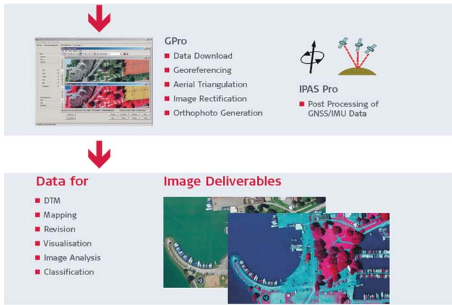
Fig. 7.1-21 Overview of the ADS40 and ADS80 Data Processing Workflow
