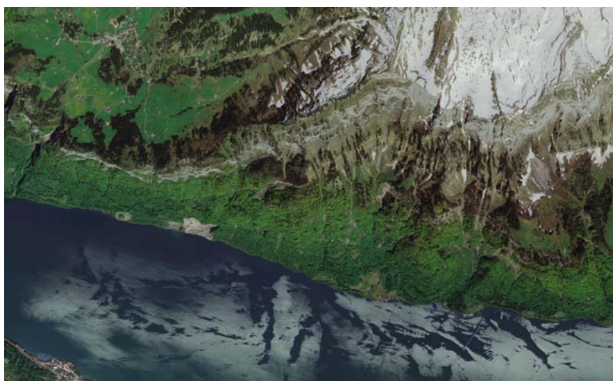
Fig. 7.1-24 Walensee, Switzerland, Orthophoto for alpine area mapping 1:5000, altitude 2.0-/3.6 km, GSD 20/36 cm
