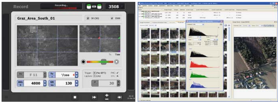
Fig. 7.3-5 COS GUI ( left ) enabling the on board quality control of each picture and OPC GUI ( right ) addressing an entire flight mission with many images
