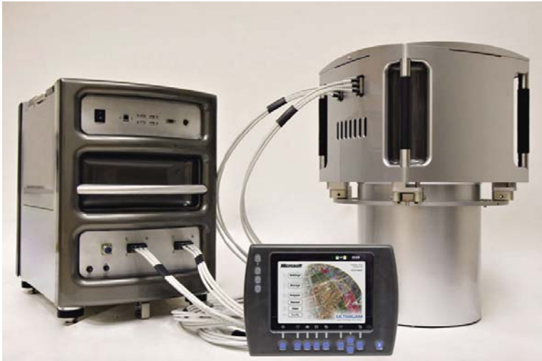
Fig. 7.3-2 The UltraCamX digital aerial camera system with the Sensor Unit ( right ) and the airborne Computing Unit including two removable Data Units ( left ). The camera is operated in the air through the Interface Panel ( middle )
