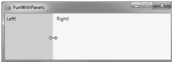
Figure 28-11. Grid types containing splitters
