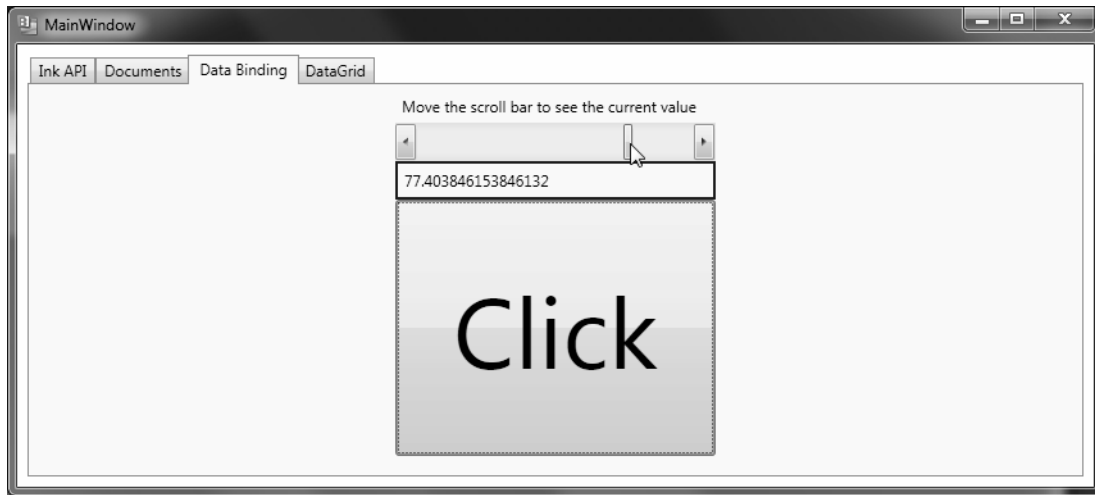
Figure 28-46. Binding the ScrollBar value to a Label and a Button
