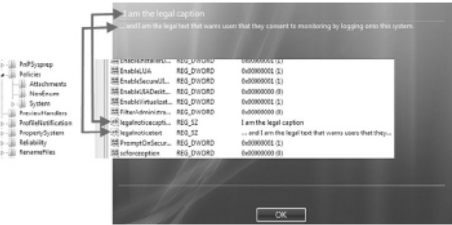
FIGURE 5.22 Registry values entered to present legal warning messages at system startup.
