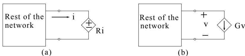
Figure C.3. Application of the substitution theorem in current- and voltage controlled dependent sources.
