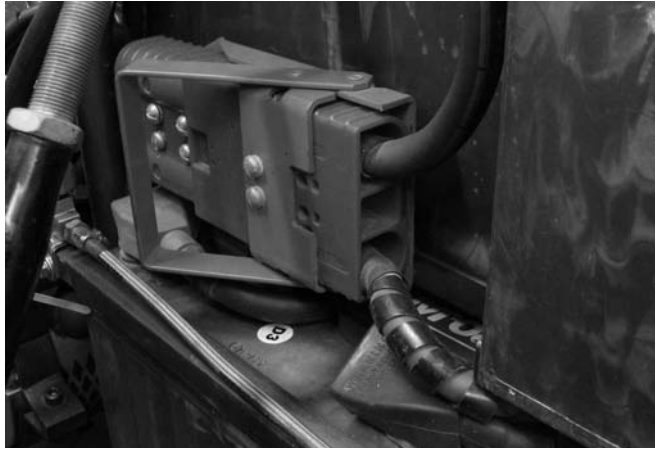
FIGURE 12-2 Quick disconnect on the Electra Cruiser.
