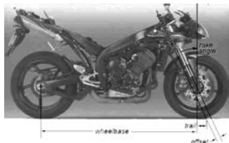
FIGURE 5-2 Picture of bike front headstock angle in relation to ground. (Courtesy of Chris Longhurst, www.carbibles.com/suspension_bible_bikes.html .)
