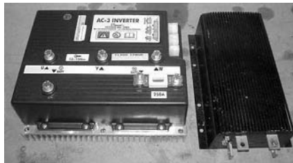
FIGURE 9-32 ZAPI AC3 ac controller size compared with the Curtis 1231.
