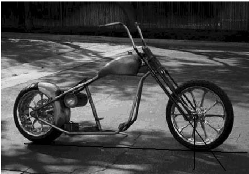
FIGURE 5-4 Rolling frame with reference lines drawn showing trail.
