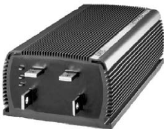
FIGURE 9-6 Curtis Model 1231C 15-kHz PWM controller.
