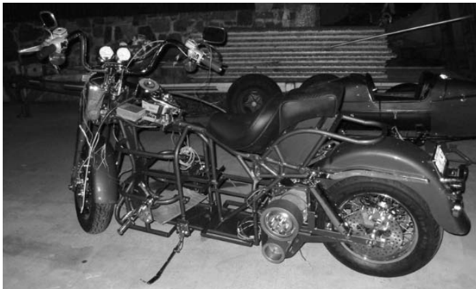
FIGURE 13-4 Prototype 2 Electra Cruiser ready for batteries.
