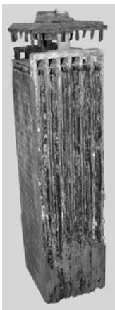
FIGURE 7-14 Sulfation of battery plates. ( www.surfacematerials.com/Cell_sediment.jpg .)
