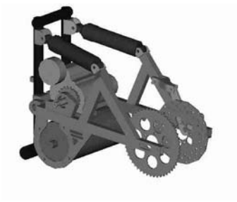
FIGURE 5-17 3D drawing of the Hybrid swingarm design: First-generation Electra Cruiser.
