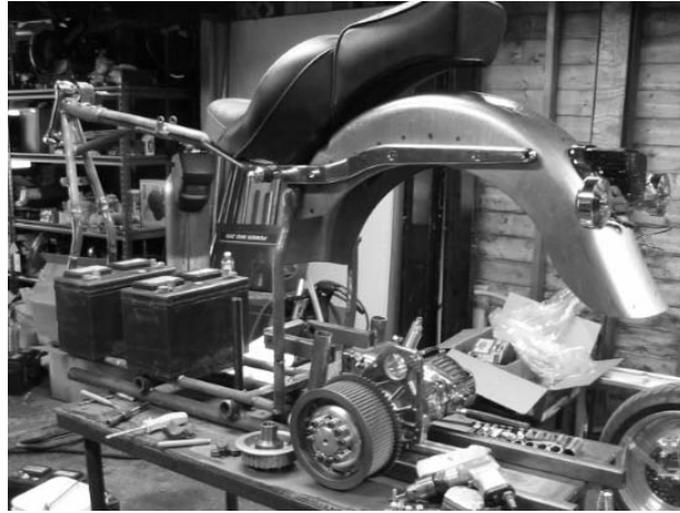
FIGURE 13-7 Fitting the transmission to the swingarm.
