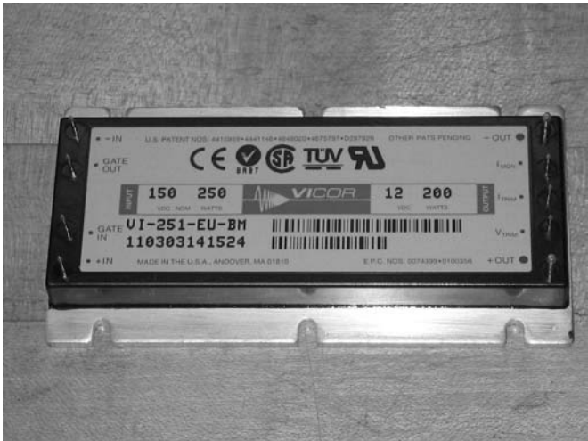
FIGURE 11-13 Vicor BatMod dc-to-dc converter.
