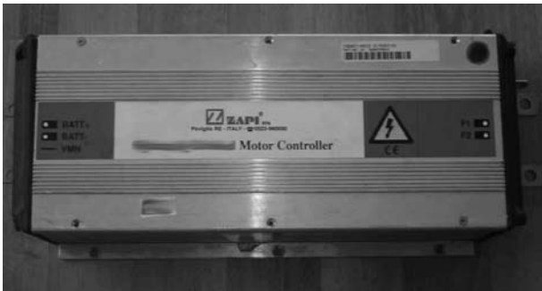
FIGURE 9-18 ZAPI dc series motor controller.
