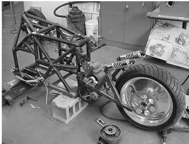
FIGURE 13-8 Transmission placed on prototype 1 swingarm.
