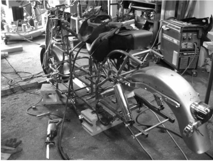
FIGURE 13-6 Prepping the Cruiser frame for cleaning and more welding.
