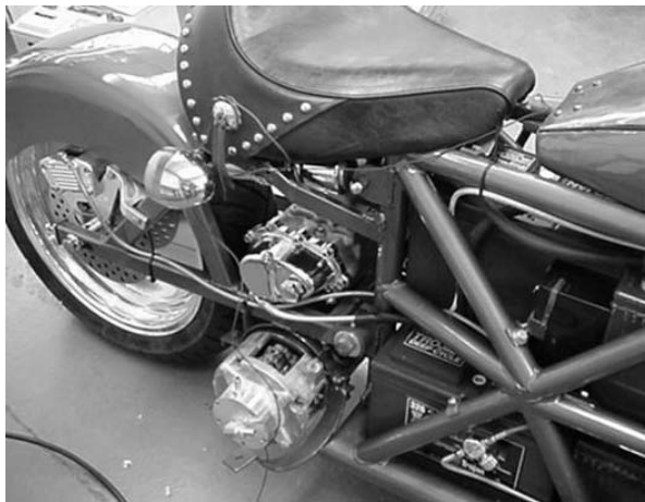
FIGURE 13-13 Rear mounting bracket for the dc motor.
