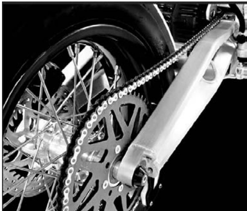
FIGURE 13-9 ZERO electric motorcycle chain drive. ( www.zeromotorcycles.com/gallery.php .)
