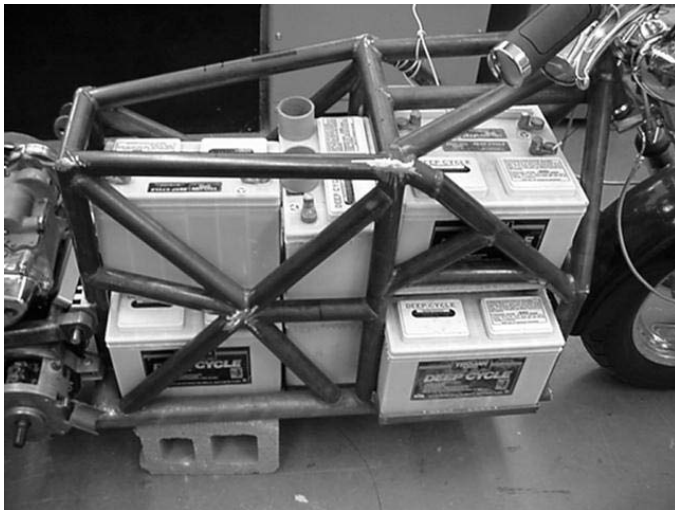
FIGURE 13-16 Fitting 10 Group 27 batteries in prototype 1.
