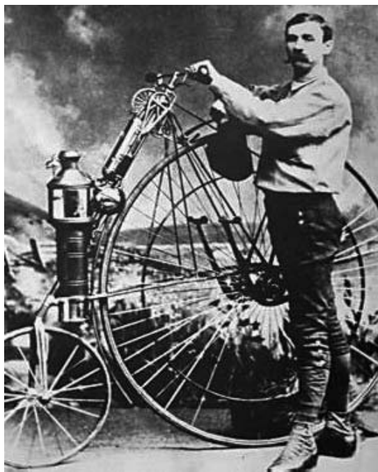
FIGURE 3-2 Another view of Lucius D. Copeland and his steam bicycle. ( http://patentpending.blogspot.com/photos/uncategorized/early_tricycle_1.jpg .)
