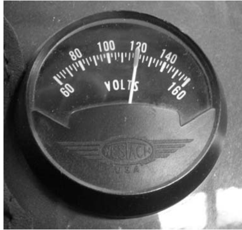
FIGURE 11-8 Voltmeter used on the Electra Cruiser. ( www.westach.com/gauge_images/2C6-30.gif .)
