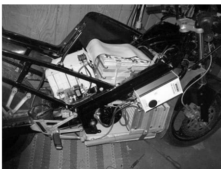
FIGURE 4-2 Electrocat batteries and electric motor. ( evahakansson.se .)
