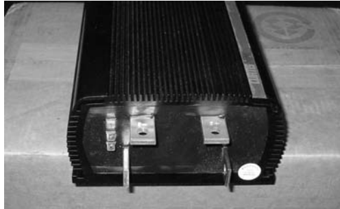
FIGURE 9-16 View of Curtis Model 1231 series connections. ( www.curtisinst.com/index.cfm?fuseaction=cProducts.DownloadPDF&file=50003%5F1221C%2D1231C%5FRevD%2Epdf .)
