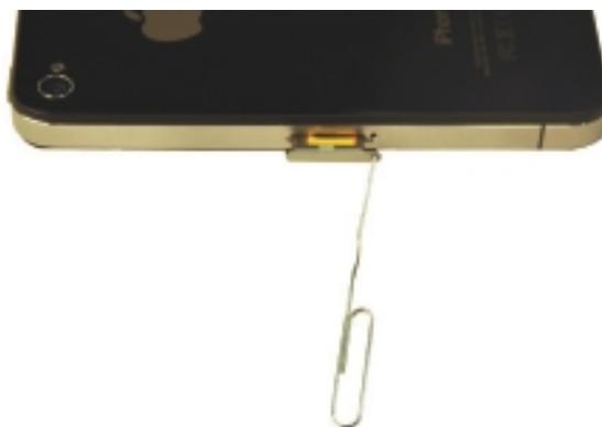
Figure 15-2: Removing the SIM tray on an iPhone 4.
