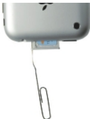
Figure 15-1: Removing the SIM tray on an iPhone 3G or 3GS.
