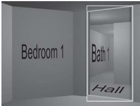
Figure 16.13: The bounding box of a portal polygon
