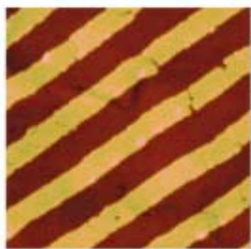
Atomic-force microscopy image (left) and 3-D rendering of DNA wires stamped on a gold substrate in process pioneered by Francesco Stellacci.
