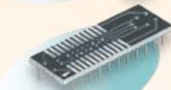
24-pin SOIC to 24-pin 0.3in. DIP
