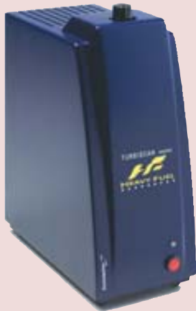
Turbiscan Heavy Fuel instrument undertakes oil stability checks in 15 minutes
