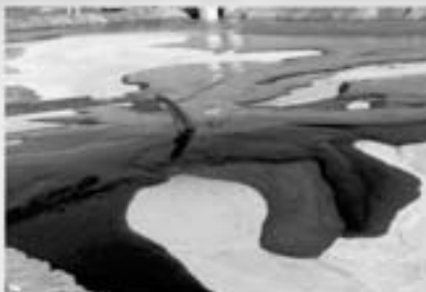
USA: high density tailings disposal
