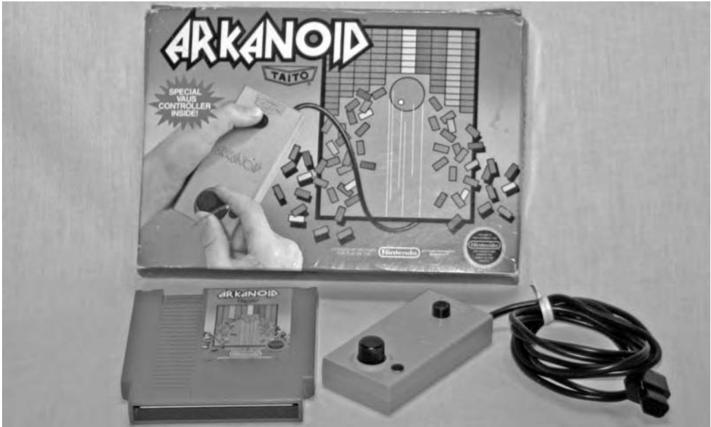
Arkanoid for the NES, with box and special “Vaus” controller, which is a rotary device similar to the Atari 2600 paddle controllers.
