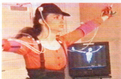
Magnetic motion capture is relatively cheap, but the wires inhibit movement
