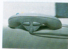
The Power Player's redesigned controller features a directional pad and a trackball, plus two shoulder buttons and four thumb buttons arranged in a diamond formation
