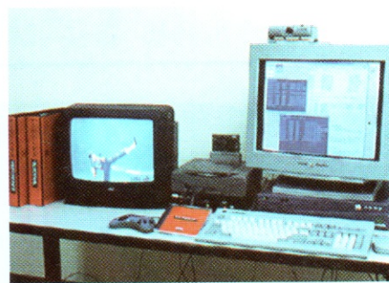
Previously, the Saturn development system included a P-Box, or programmer box (left), instead of a production Saturn. In the new system the P-Box has been replaced by SOA's CartDev box, which sits below the Saturn, and a cartridge which interfaces with the PC or workstation. Sega's 'official' development set-up (right) includes an SGI Indy, Softimage, CartDev, SNASM2, and AM2's SGL
