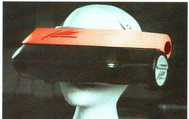
KaiserOptics' Vision Immersion 1000 , the larger brother of the VIM 500 used in Hasbro's Onyx-based development kit. The final system is reported to feature a headset with a built-in microphone
