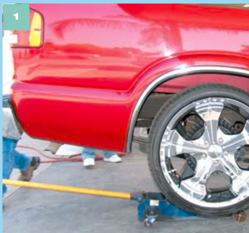
With the rear-end raised off the ground, and safety stands under the axle with wheel chocks in place, remove the rear wheels. Assemble the upper bracket with the swivel air fitting facing towards the front of the truck.
