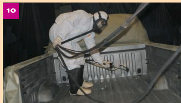
The operator uses an applicator gun that applies the Rhino Linings mixture to the bed. It is applied like paint and the operator can add various layers to increase the thickness of the application.
