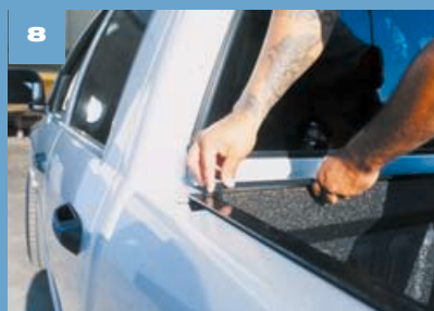
He then mounts the drip trail by securing the mounting tabs, affixing the mounting brackets, and compressing the bottom foam seal so he can tighten the mounting nuts.
