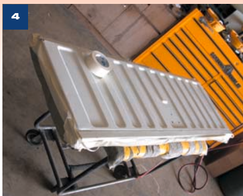
4 Tailgate's exterior is protected and only the surface that receives the spray-in liner is exposed.
