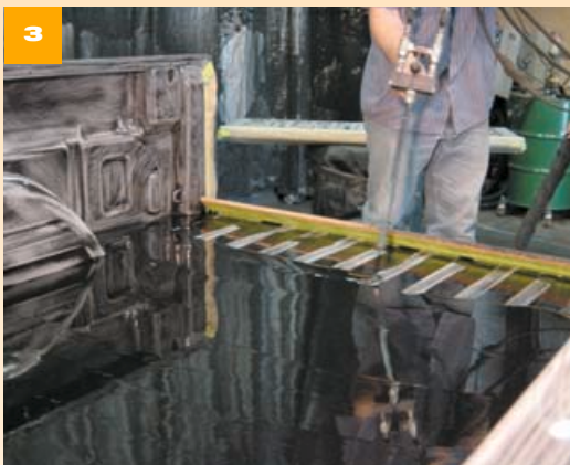
The Fabick liner is poured to completely fill the floor of the bed and it will form a thick coat that will protect the sheet-metal from heavy-duty use.
