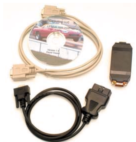
This is what we received from Carputing to reprogram the Sierra's ECM. This, via a laptop, allows us to reprogram any aspect of the vehicles system including all transmission functions as well as the engine.
