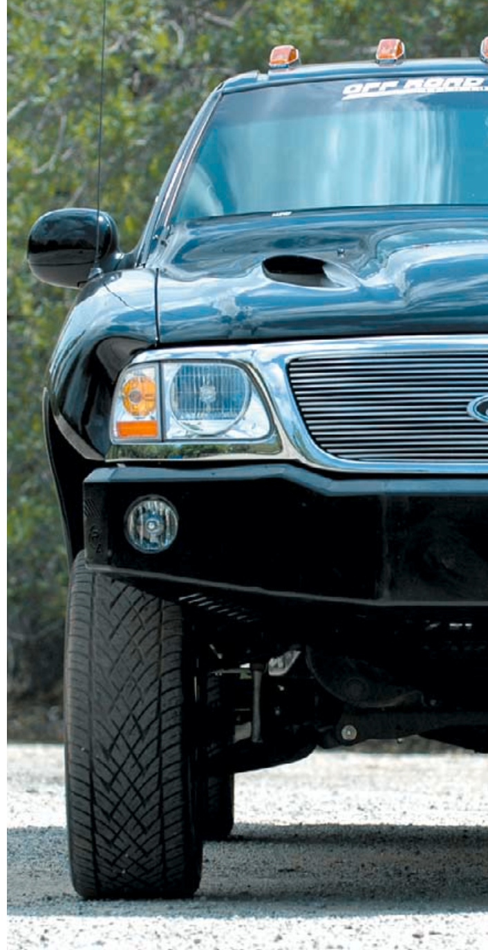
Sporting a 6-inch lift and Road Armor bumpers, the F-150 has the ground clearance of a real pre-runner truck.
