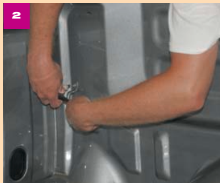
2 Items such as the cargo cleats are removed to avoid overspray. These will be reinstalled after the liner is applied.
