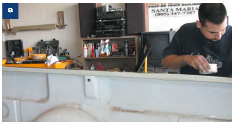
8 Once the drop-in bedliner is removed, the bedrails are masked off. Late model Ford trucks have a more permanent plastic top rail protector, so it is more logical to leave it in place. Other trucks lend themselves more readily to the extending of the Line-X coating over the top bedrail.
