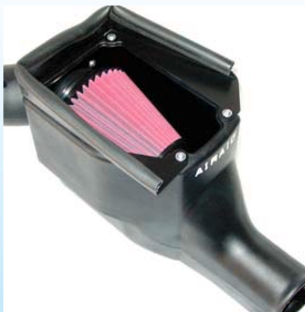
1. Airaid's intake system for the '03-'05 Ford Power Stroke Diesel is a complete replacement setup that utilizes the factory air inlet location and has provisions for the OE mass air meter.
