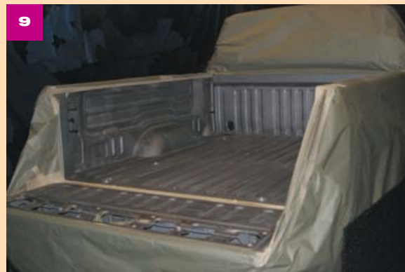
This is what the bed of the truck looks like, fully scuffed, masked, and ready for the application of the urethane liner.
