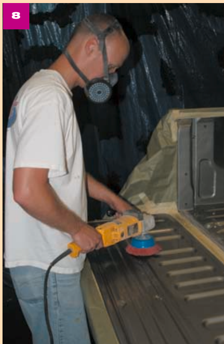
The larger areas of the bed are scuffed using an appropriate brush to merely scrape the paint enough for proper adhesion.
