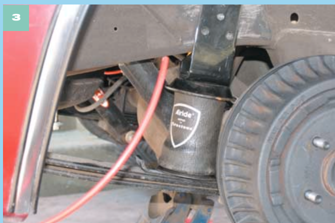
Set the entire lift assembly on the leaf spring. Make sure the air fitting is pointed forward and that the entire upper assembly is parallel and perpendicular to the lower bracket. Holes are provided so you can drill and bolt the assembly to the truck frame. As you can see, this install was welded.
