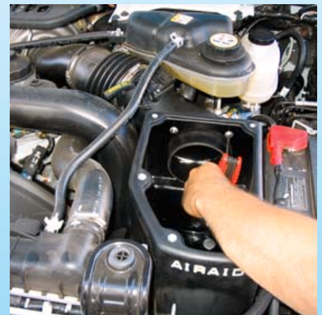
10. With all the sensors mounted to the intake tube, the assembly can be installed in the truck as per the instructions.
