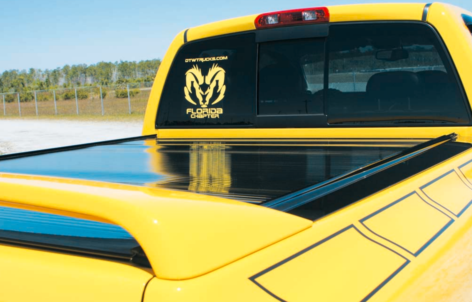
Line-X bedliner and a Retrax roll-top bed cover finish out the truck bed.
