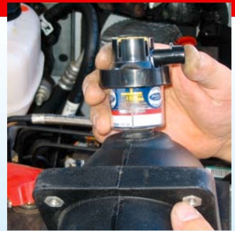
9. The factory filter minder was also re-installed on the new intake.
