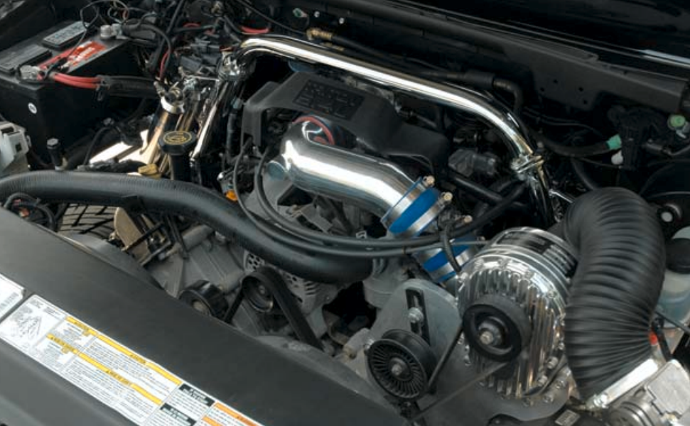
The 5.4-liter V-8 was augmented with a Powerdyne supercharger and a Borla cat-back exhaust system.
