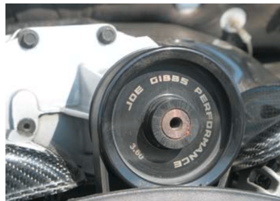
Even the supercharger pulley has the Joe Gibbs name on it, and yes, you could probably install a smaller diameter pulley to make more boost.
