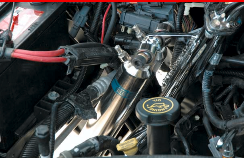
▲ Because the truck was only lifted six inches, ORU had to fabricate custom shock hoops to fit the Bilstein 7100 series shock absorbers.
