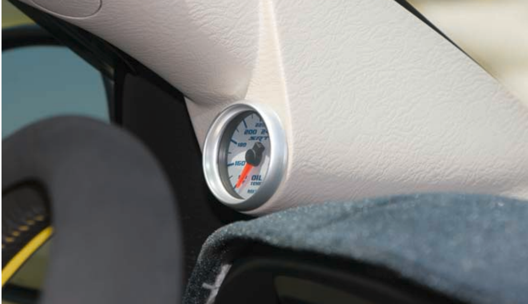
White faced A-pillar oil temperature gauge gives the eyes one more thing to look at.
