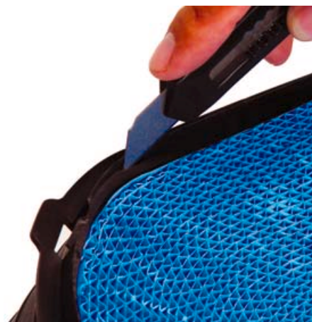
Using a cutting tool, carefully separate the filter element from the housing.
