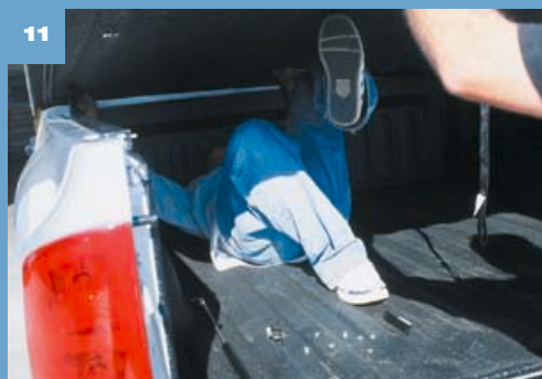
Reclining beneath the closed lid, the installer affixes the gas props to the prop balls on the framerrails while the lid is lifted slightly.
