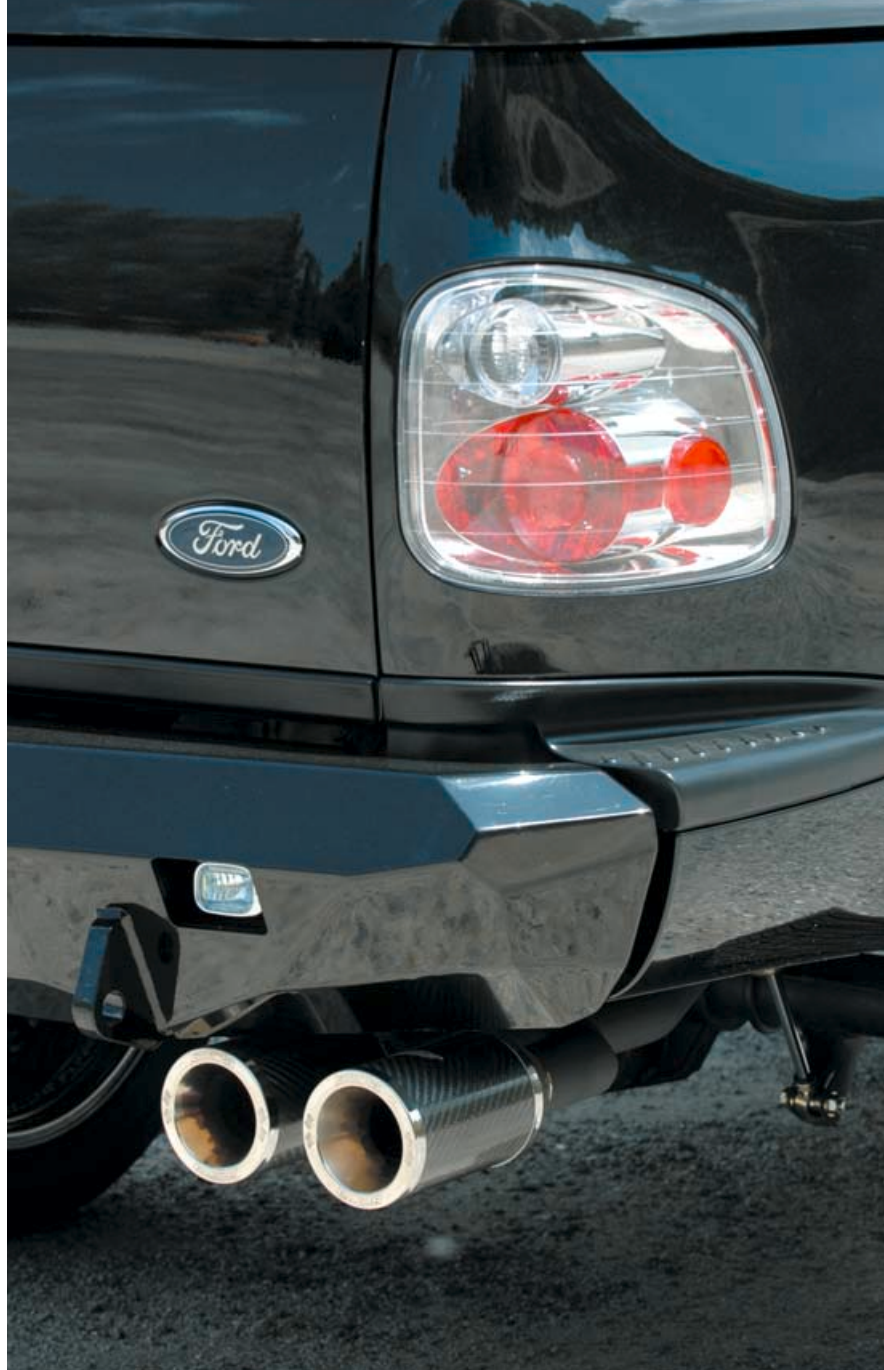
Lightning taillights and headlights were used and the Borla exhaust system protrudes from under the Road Armor bumper with a carbon fiber tip.
