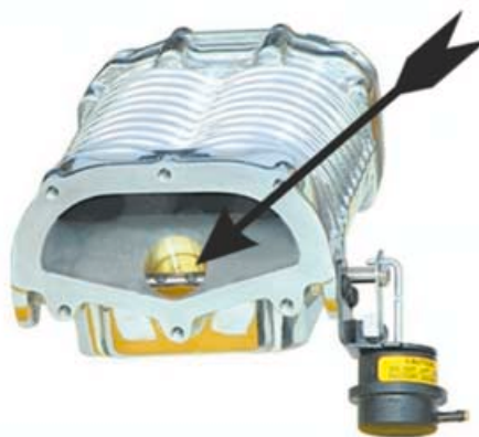
The low parasitic losses produced by the Eaton/MagnaCharger are the result of the addition of this bypass valve.
