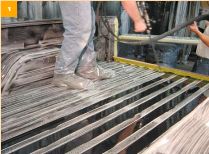
The Fabick liner is applied in several stages. First, the truck bed is sanded and prepped just like most urethane liners. The truck is then placed on a level surface and all of the drain holes and seams are caulked. Then the edge of the bed is dammed-off and the Fabick urethane product is poured to fill between the bed floor corrugations.
