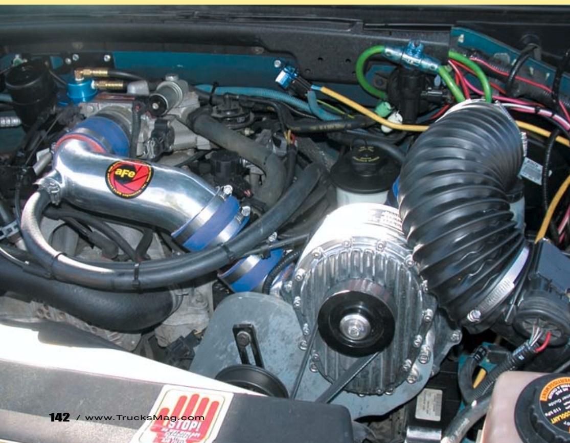
A Powerdyne centrifugal supercharger wakes up the 4.6-liter Triton motor. Gibson headers and mufflers route exhaust out.
