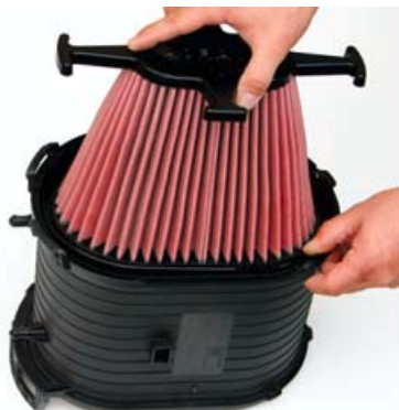
The new AIRAID Premium Replacement Filter simply slides down inside the stock canister.
