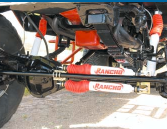
A Dana 60 straight axle suspended with eight-inch springs work with Rancho steering stabilizers and shocks. That's a Moroso deep sump oil pan your eyeballing at the bottom of the big-block. All suspension parts were painted with tool black.
