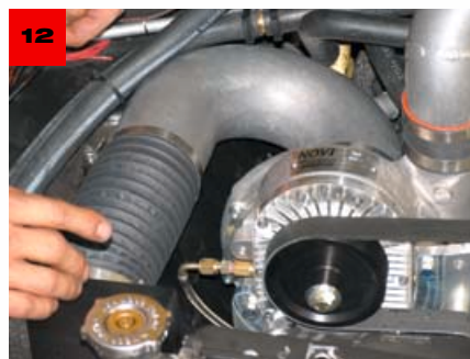
Install the ducting tube from the supercharger to the air-cleaner box.
