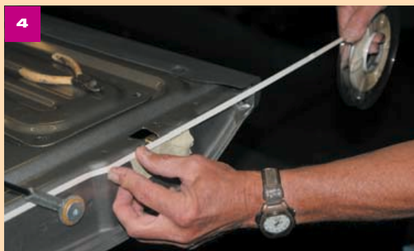
4 Wire tape is used on some of the exposed edges. This allows the urethane to have a clean-cut edge when the masking is finally removed.
