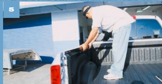
Cleverly designed, built-in clamps are tightened to affix the framerrails securely to the truck bedrails. This way, no drilling is necessary.
