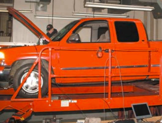
Here we are just about to start testing on More Performances above ground, Dynojet chassis dyno after the head install. Peak power rose from 242 hp to 262 at the rear wheels.
