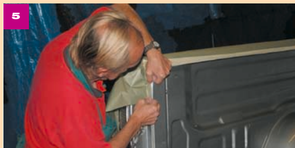
5 The rest of the truck is masked to avoid any urethane liner overspray onto the rest of the truck.
