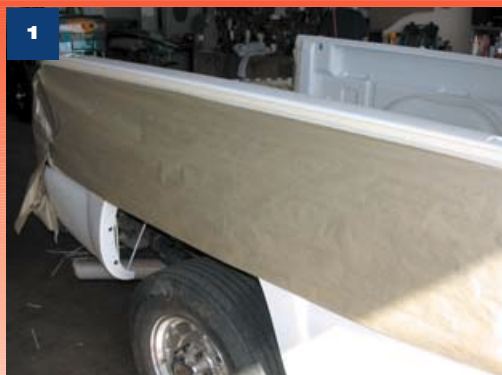
1 Truck bedsides are protected with construction paper and plastic.
