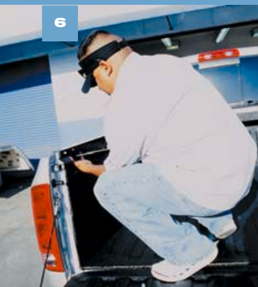
The installer removes the framerrails and unties the gas props, which were secured to the lid for shipping.
