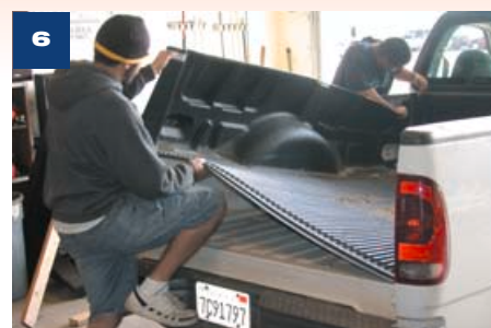
6 Once freed, the entire drop-in bedliner is removed.
