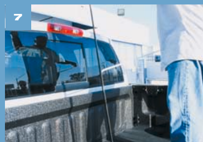
Our installer gets ready to install the drip trail by first peeling the protective strip from the adhesive backing.
