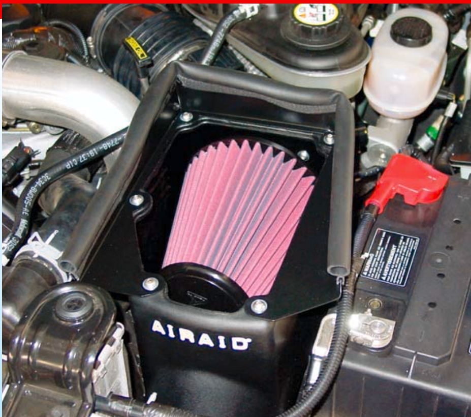
12. The finished install not only looks factory, but it's good for an additional 21.2 rear-wheel horsepower and improved throttle response from the big turbo diesel.
