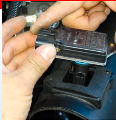
8. The OEM mass air meter was carefully replaced on top of the AIRAID intake using the supplied gas-ket
