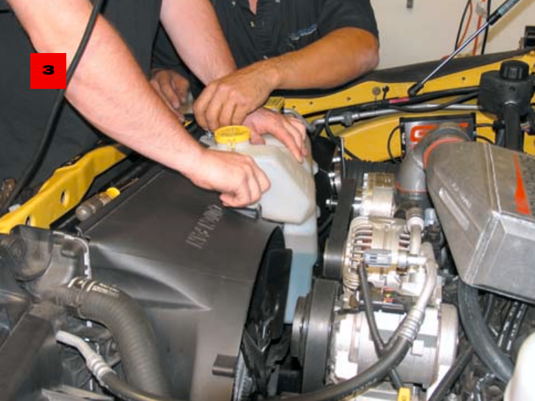
Reinstall the radiator overflow tank and washer assembly.
