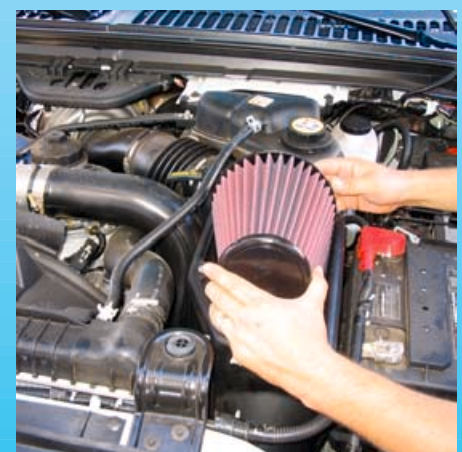
11. One of the final steps in the installation of the SynthaFlow, high-flow air filter and the sealing gas-ket on top of the Cool Air Dam.
