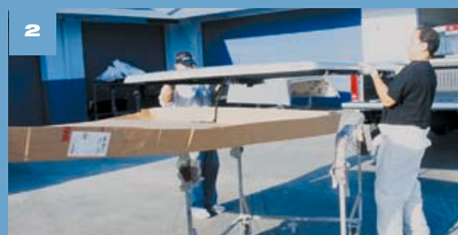
2 SnugTop color matches the tonneau to your truck's color code and it is delivered in a shipping carton. To install, the technicians at SnugTop placed it on a rack to be prepared for installation.
