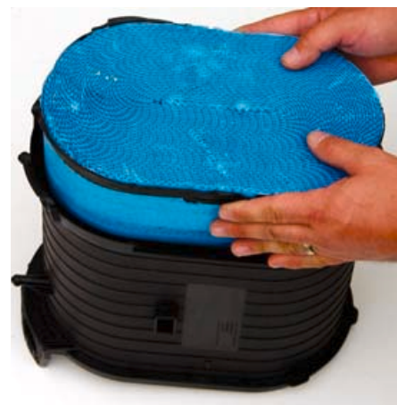
Next, remove the factory element from the housing and discard.
