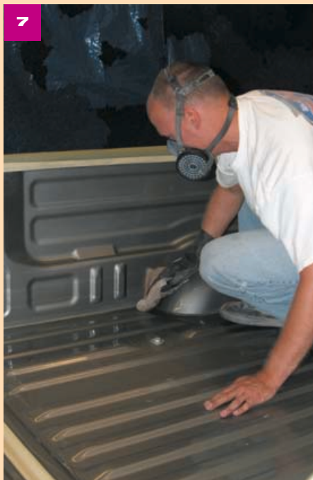
The area is then cleaned with a solvent to ensure that there is no grease or residue on the surface of the bed.
