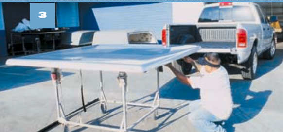
The installer removes the framerrails and unties the gas props, which were secured to the lid for shipping.
