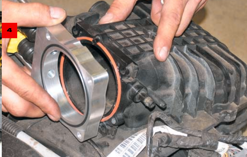
With the throttle body disassembled according to instructions, you will install the supercharger injector plate between the throttle body and the manifold with the O-ring facing the throttle body.
