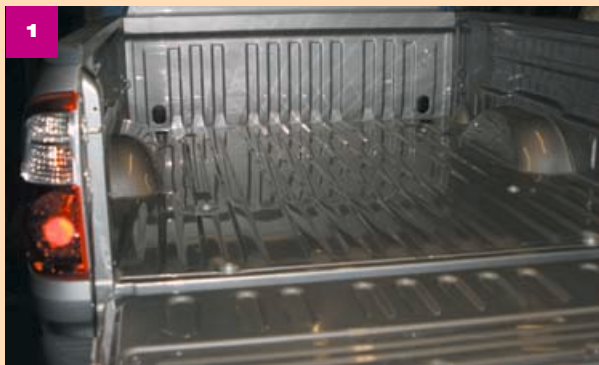
1 This stock Toyota Tundra is being prepped for a color matched Rhino Linings bedliner. The operator will mix the semi-metallic pigment into the urethane mix to closely match the truck's exterior paint.
