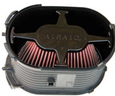
The finished install should look like this. Re-assemble the canister containing your new AIRAID Premium Filter back into the factory intake system.
