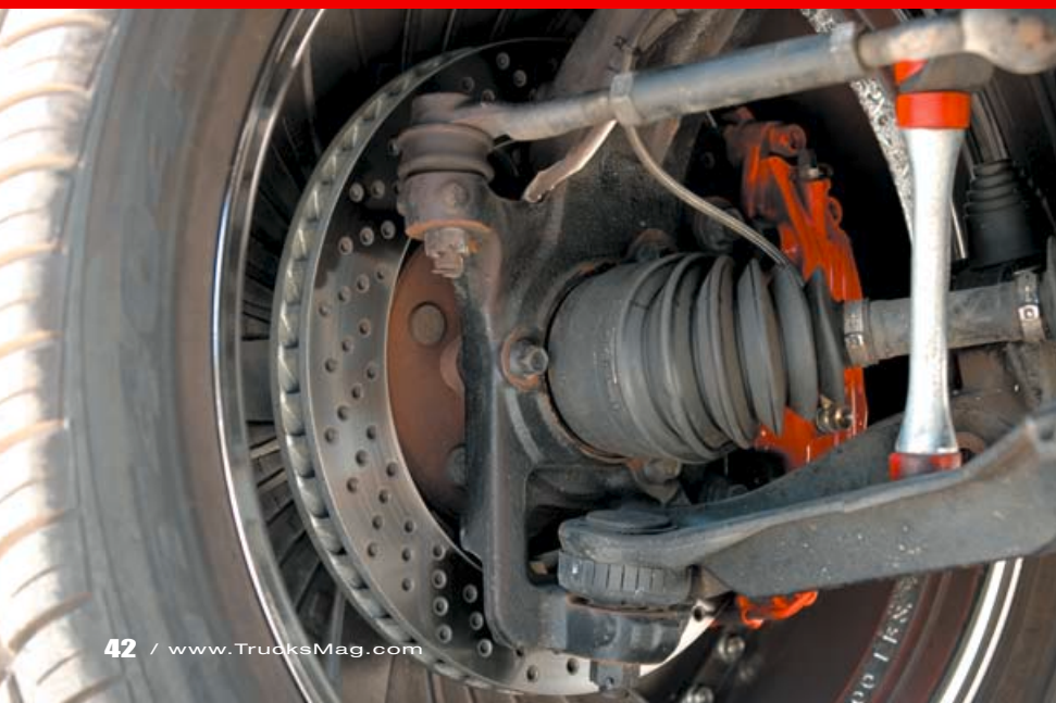
▲ Because the truck was only lifted six inches, ORU had to fabricate custom shock hoops to fit the Bilstein 7100 series shock absorbers.
