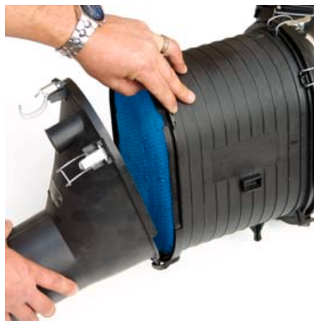
The first step of the install is to unclamp the factory filter element from the housing. For photo purposes, the entire intake setup was removed from the truck for better viewing.
