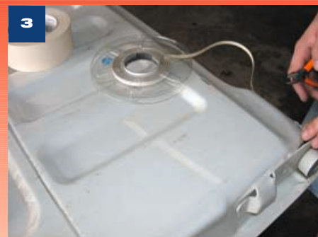
3 Detail tape outlines the area to be sprayed. After the Line-X is applied, and the protective masking plastic comes off, the fine wire embedded in this white tape will be pulled and it defines the clean separation between paint finish and the protective liner.
