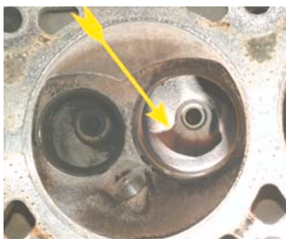
GM did not form that bulky guide boss just to use up aluminum. It's there to generate certain swirl characteristics necessary for improved low-speed torque and better emissions. The characteristics it develops must be preserved when porting these heads.
