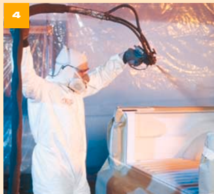
The Fabick urethane product is sprayed on with a high-pressure system that covers the rest of the bed including the floor, and the bed floor is left to dry completely. This applies a non-skid finish and also protects the sides of the bed.
