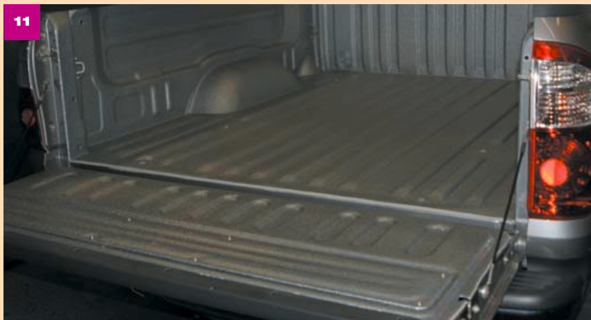
The result, after the masking is removed, looks great and almost perfectly matches the exterior color of the truck's paint. A UV topcoat was also applied to ensure that the color does not fade over time.
