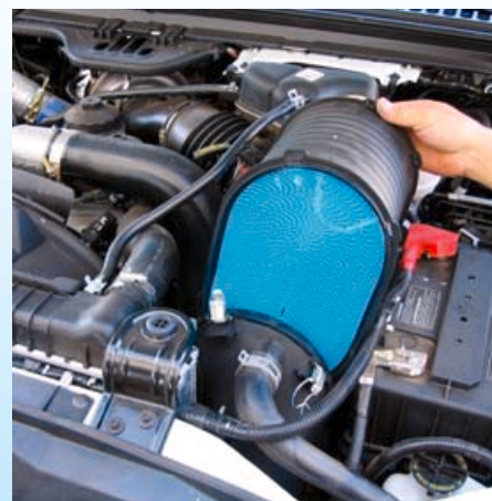
3. The install begins by removing the stock filter element.
