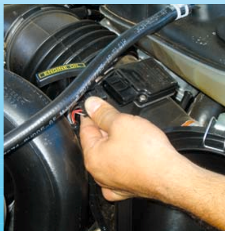
5. Next, the wires connected to the factory mass air meter are unplugged.
