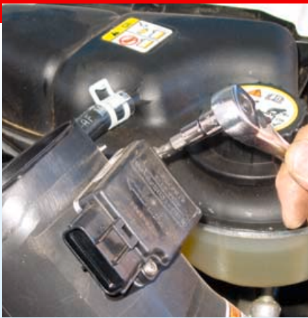
7. The AIRAID intake kit includes a special bit to remove the factory mass air meter from the original housing.
