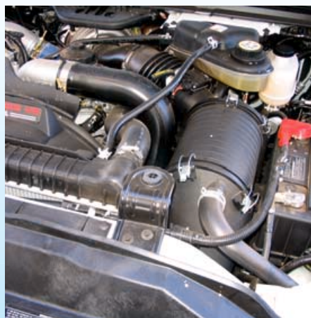
2. The stock air intake system utilizes a rather large filter that sits inside a plastic housing on the driver's side of the engine bay.
