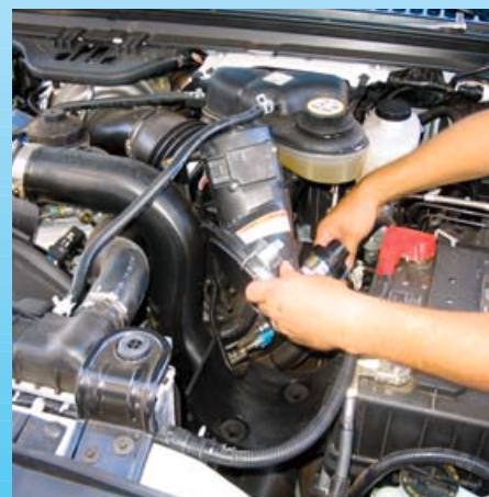
6. Next, the rear section of the factory intake housing is unbolted from the flexible ducting and removed. The factory filter minder should be saved. It will be used on the new intake.
