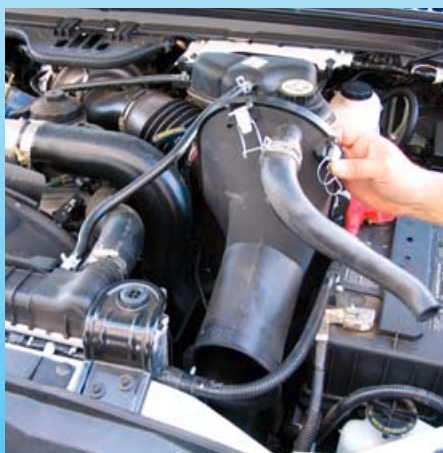
4. With the element housing removed, and hoses disconnected, the front half of the factory intake was pulled from the radiator core support.
