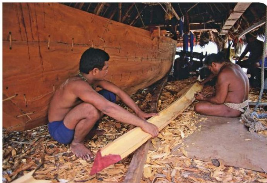
Micronesian boat builders on Satawal Island still construct sailing canoes. The hull's planks will be bound together with coconut-fiber cords.
