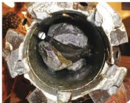
Volcanic material called basalt is shown here inside a research vessel's drill core.
